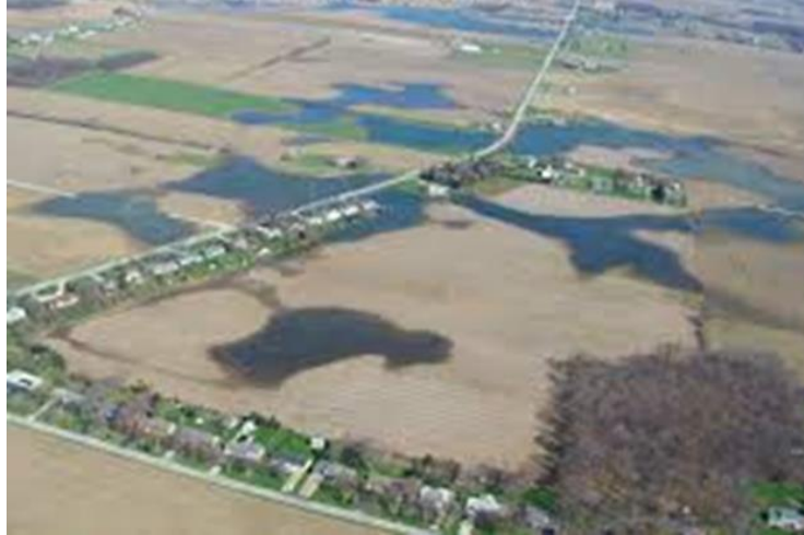
Figure 3-3: Internally drained sinkholes with pooling in Bellevue, Ohio
