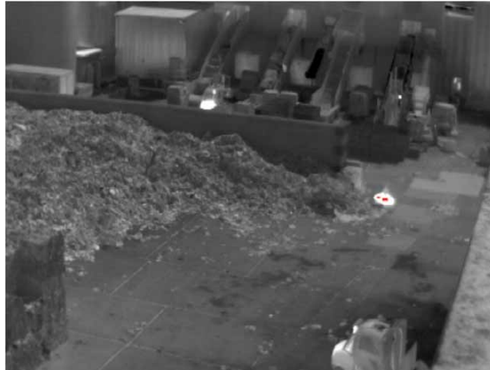
Figure 9: Passive Thermography for Long Range Fire Detection (Dias – Infrared Systems)
