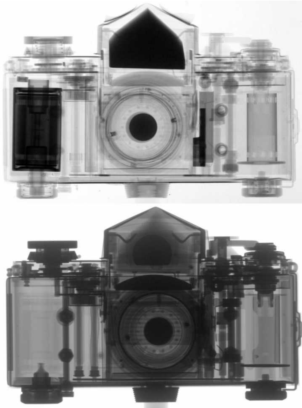
Figure 1.2: Top: neutron radiograph of an analog camera. Film can be seen to the left and right of the lens. Bottom: the same camera imaged with x-rays. Figure from [2].
