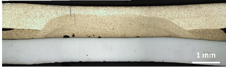
Figure 5.22 Macrostructure of Al/steel welds using U+RSW with a dome-shaped electrode on the steel side (welding current of 19 kA, welding time of 67 ms, and MFDC machine)
