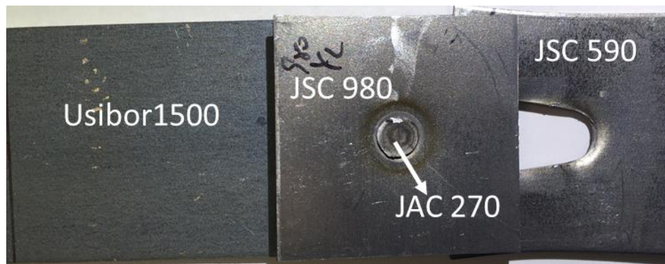
Figure 4.41 Button pull-out on JAC270 during peel test and button pull-out from JSC 590 during lap-shear tensile testing
