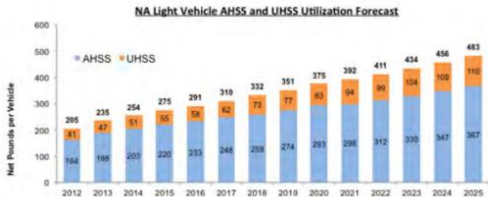
Figure 2.1 Net weight of AHSS and UHSS per NA light vehicle (2012 – 2025) [1]
