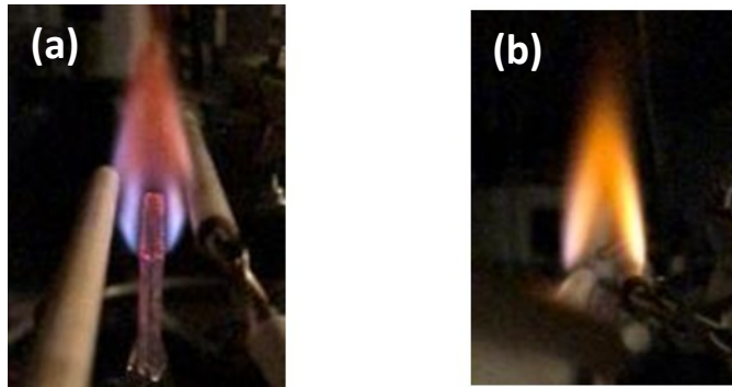
Figure 5.12. Photographs of a hydrogen diffusion flame for different gaps between the electrodes: (a) d = 12 mm, flame is attached to the flame spreader exit; (b) d = 4.5 mm, flame is attached to the top of the electrode sleeves. In both cases, electrode sleeves are placed 2 mm above the flame spreader exit. Hydrogen flow rate 1 SLM, no plasma.
