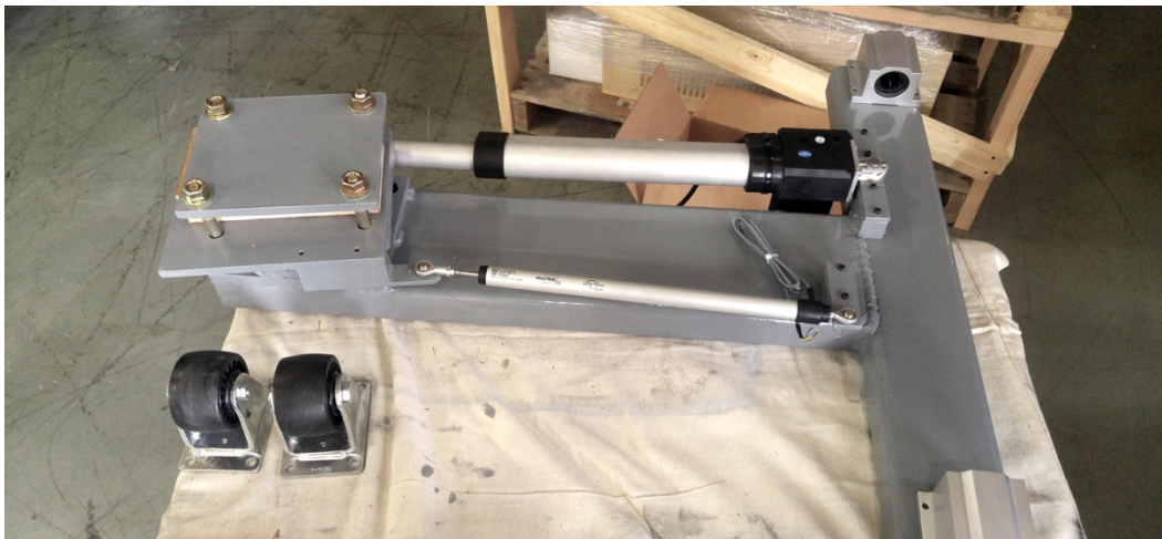
Figure 40: Sliding Seat Support Construction
