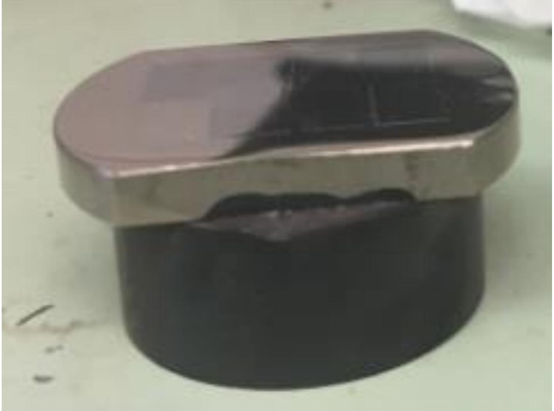
Figure 16. Photo of the polished Co-Cr-Fe-Mo-Ni diffusion multiple sample after being assembled, HIPed and heat treated. The sample was glued to a bakelite mount for experimental convenience.
