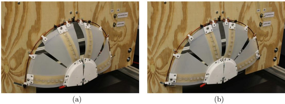
Figure 8.16: (a) Unactuated domed shape and (b) actuated flat shapes of a half-scale morphing fender skirt demonstrator.
