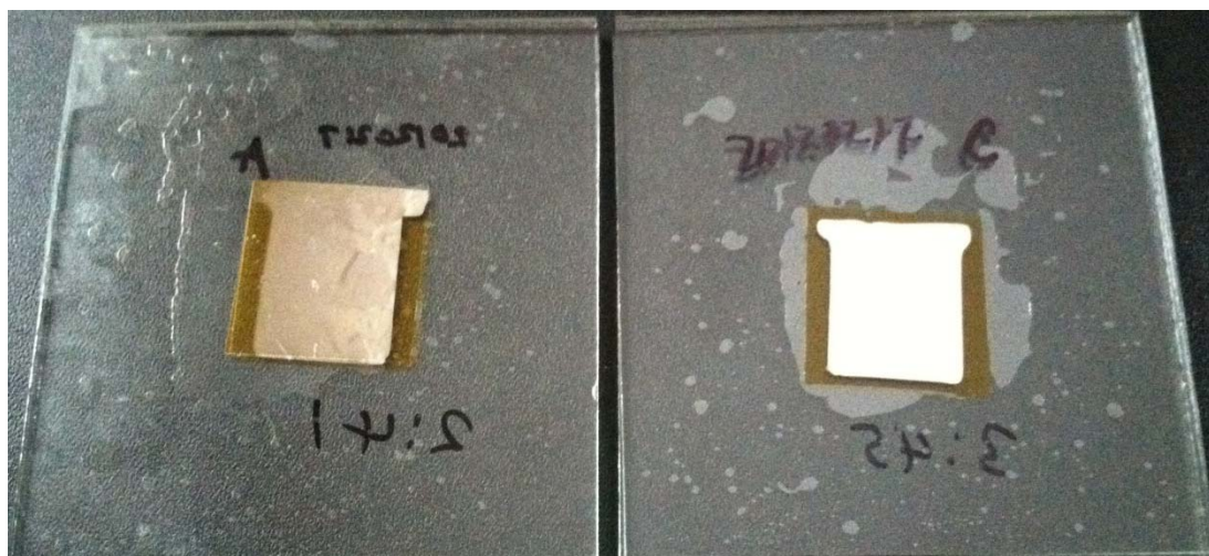
Figure 18. Composite sealing structure after 1960 hours exposure to ambient air, left: prototype sealant A and right: prototype sealant C. The T-shaped calcium layer (metallic shiny) appears grey on the left and white on the right in this photo.
