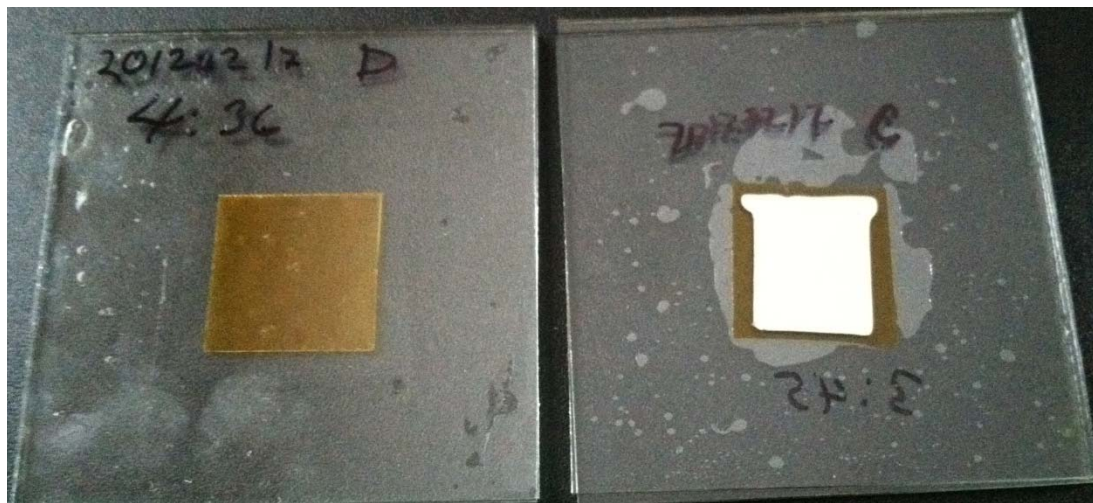
Figure 17. Composite sealing structure after 1960 hours exposure to ambient air, left: PDMS control sample and right: prototype sealant C. Note that calcium was completely corroded in the structure sealed with PDMS control sample in 22 to 24 hours, as evidenced by complete “exposure” of the amber-colored polyimide film underneath the transparent calcium hydroxide. The T-shaped calcium layer (metallic shiny, but appears white in this photo) is shown on the right.
