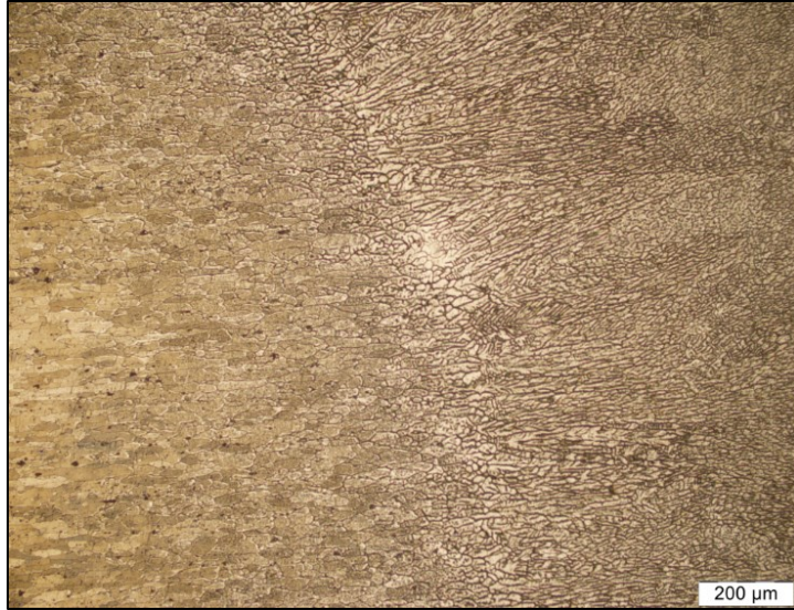
Figure (3.30): Optical microscope picture with transverse view showing the result of fast weld process of the fusion boundary with average grain size of (12.5 μm).
