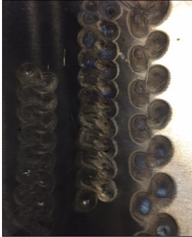
Figure (4.2): Showing three different resulted tandem weld trails for three different start hold times and two different weld travel speeds, on the right a start holding time of (4 seconds) and weld travel speed of (4.2 mm/s), in the middle a start holding time of (6 seconds) and weld travel speed of (3.6 mm/s), and on the left a start holding time of (4 seconds) and weld travel speed of (3.6 mm/s).
