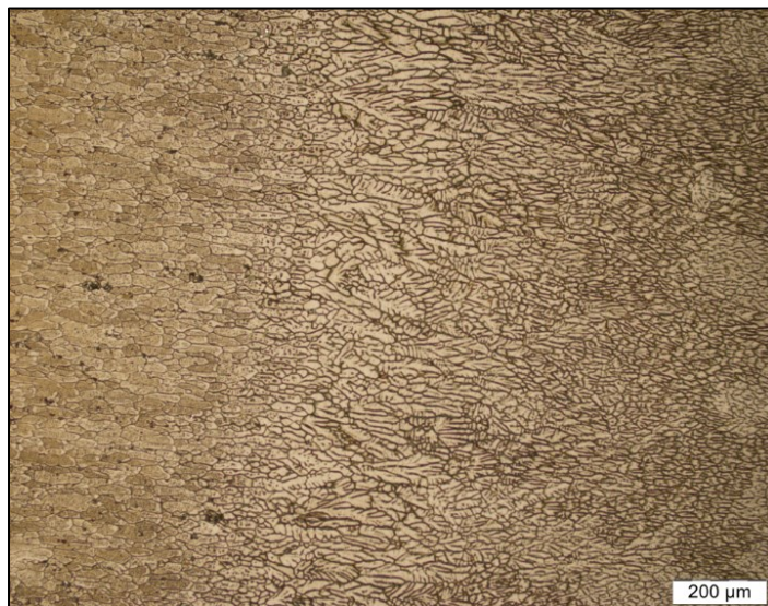
Figure (3.29): Optical microscope picture with transverse view showing the result of slow weld process of the fusion boundary with average grain size of (21 μm).
