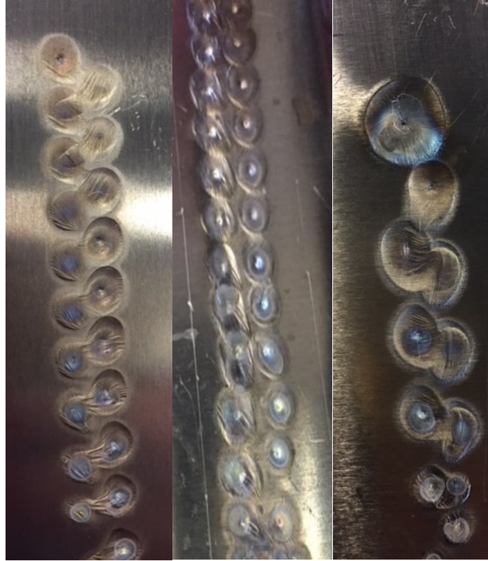
Figure (4.1): Showing three different resulted tandem weld trails for three different working times for each electrode, on the left (0.5 second), in the middle (0.75 second), and on the right (1 second). All the trails made by (3.6 mm/s) weld travel speed.
