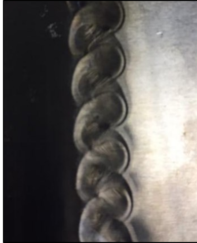
Figure (4.3): The best weld obtained by tandem weld process with a start hold time of (4 second), working time for each electrode of (1 second), and weld travel speed of (3.6 mm/s).
