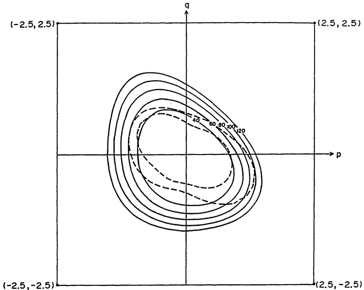
Fig. 4.14 Constant resistive force (moment), in Newtons (Newton-Meters), contour map on the modified joint axis system, in radians, for subject No. 3. The maximal voluntary hip complex sinus (inner dashed) and the maximal forced sinus (outer dashed) are also indicated.
