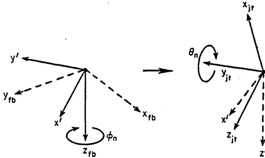
Fig. 3.10 Joint axis system as obtained by two successive rotations, first about the  $z_{fb}$ -axis and then about the intermediate (primed)  $y'$ -axis from the fixed body axis system.
