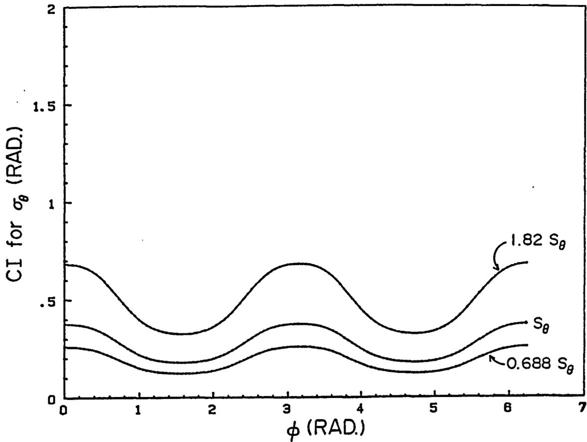
Fig. 3.20 The 95% Confidence Interval (CI) for the population standard deviation,  $\sigma_{\theta}$ . The subject-based sample standard deviation,  $S_{\theta}$ , is also shown.
