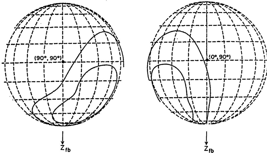
Fig. 4.16 Globographic representations of the maximal voluntary (inner curve) and forced (outer curve) sinuses for subject No. 1.
