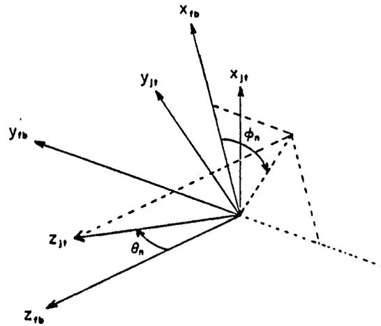
Fig. 5.3 Relative orientation of the fixed-body ( $x_{fb}$ ,  $y_{fb}$ ,  $z_{fb}$ ) and the locally-defined joint ( $x_{jt}$ ,  $y_{jt}$ ,  $z_{jt}$ ) axis systems.
