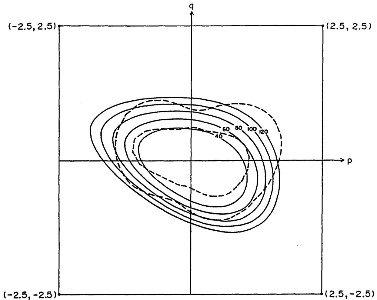
Fig. 4.13 Constant resistive force (moment), in Newtons (Newton-Meters), contour map on the modified joint axis system, in radians, for subject No. 2. The maximal voluntary hip complex sinus (inner dashed) and the maximal forced sinus (outer dashed) are also indicated.
