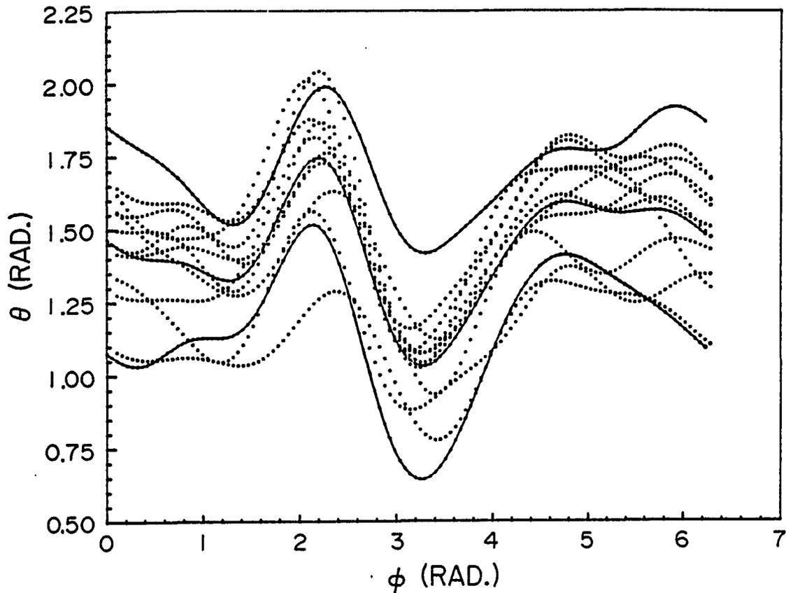
Fig. 3.14 Least-squares fitted data (dotted lines) for the space-based sinuses for all ten subjects. The middle solid curve is the space-based sample mean joint sinus  $\bar{\theta}(\phi)$ . The upper and lower solid curves are  $\bar{\theta}(\phi) + S_{\theta}(\phi)$  and  $\bar{\theta}(\phi) - S_{\theta}(\phi)$ , respectively.
