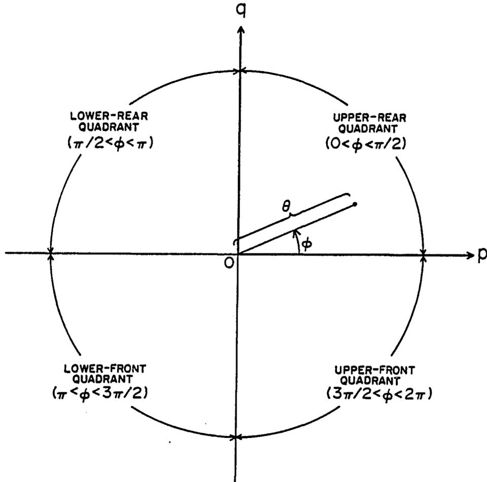
Fig. 3.6 The modified joint axis system and the corresponding four test quadrants.
