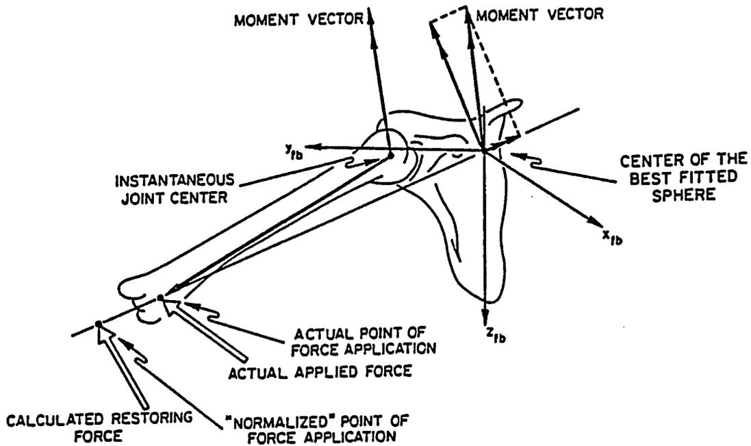
Fig. 3.5 Illustration of the vector quantities used in the calculation of resistive force values.
