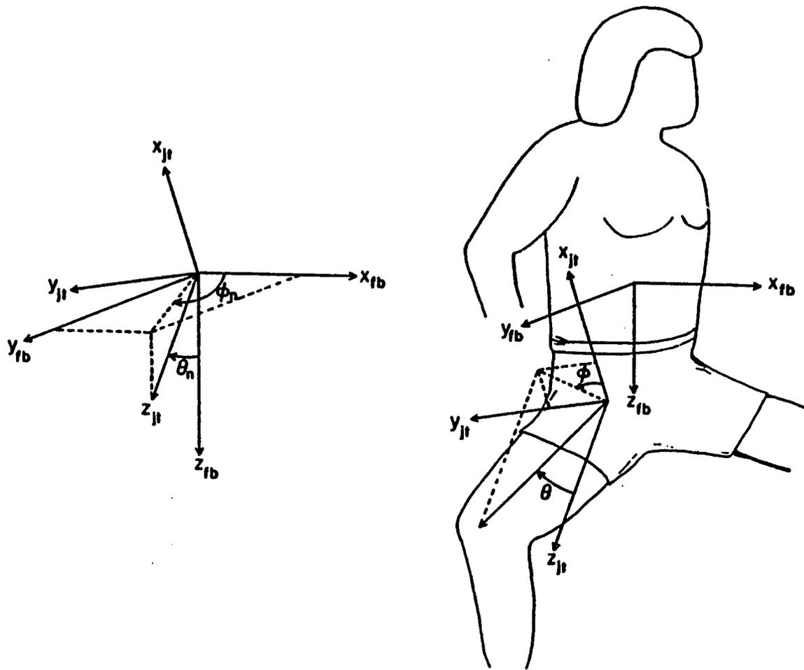
Fig. 4.3 Relative orientation between the fixed body ( $x_{fb}$ ,  $y_{fb}$ ,  $z_{fb}$ ) and locally-defined joint ( $x_{jt}$ ,  $y_{jt}$ ,  $z_{jt}$ ) axis systems.
