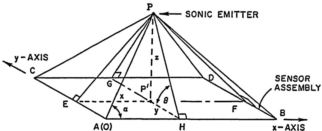
Fig. 2.1 Quantities used to convert slant range distances (PA, PB, PC) to Cartesian coordinates (x, y, z)
