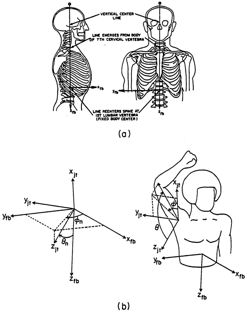
Fig. 3.2 (a) Selected origin and axis system  $(x_{fb}, y_{fb}, z_{fb})$  of the fixed segment (torso).
