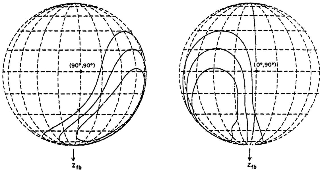
Fig. 4.20 Globographic representations of  $\bar{\theta}$  and  $\bar{\theta} \pm S_{\theta}$ .
