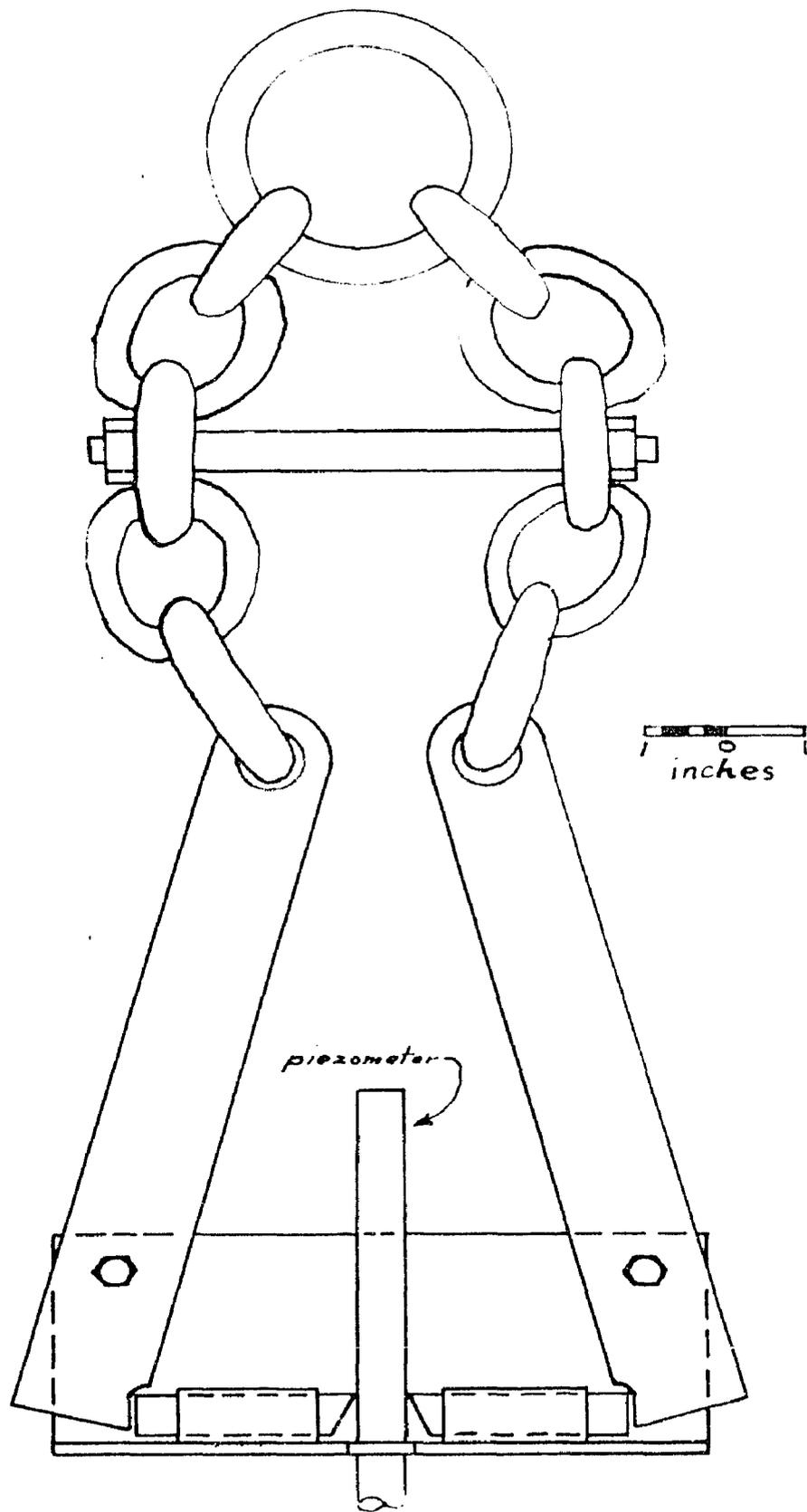
Fig. 2. Sketch of device for pulling piezometers
