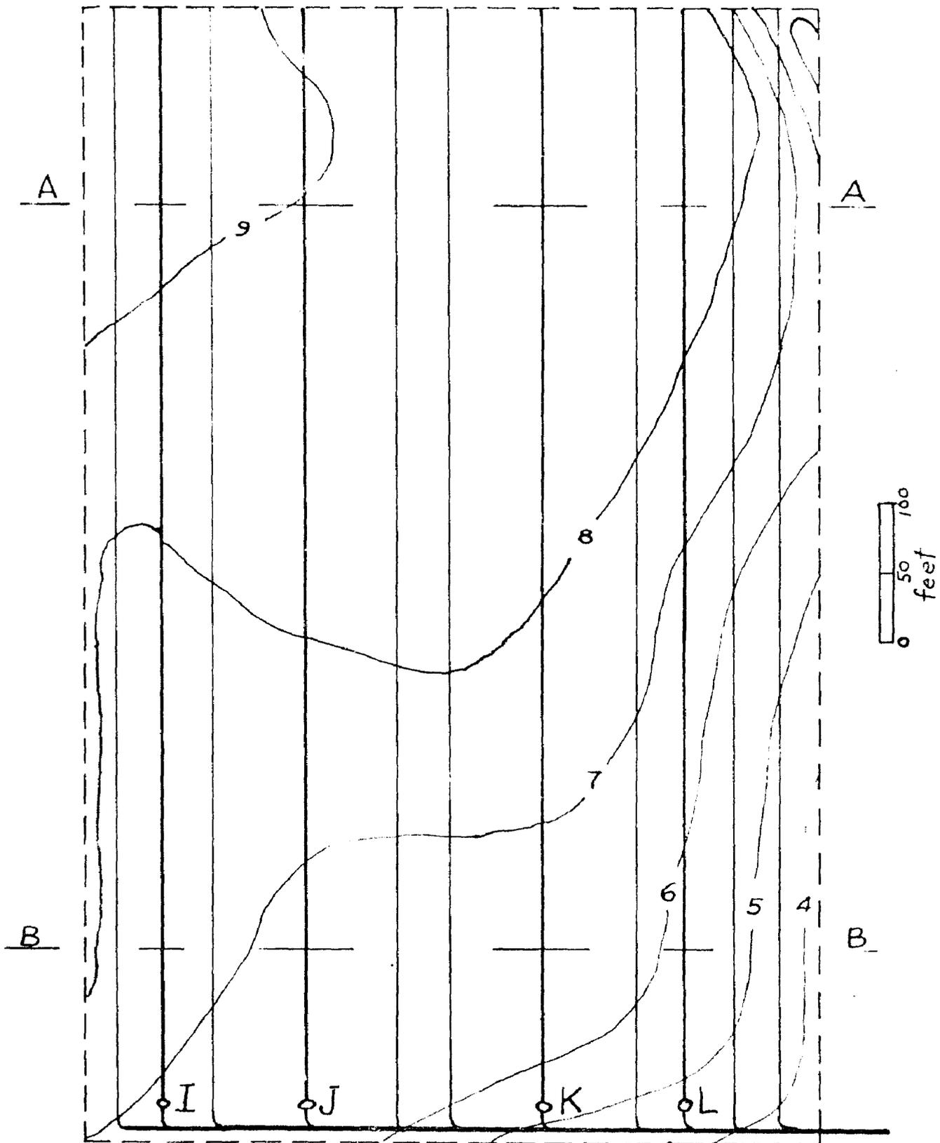
Fig. 1. Tile layout and field arrangement used for flow pattern study.
