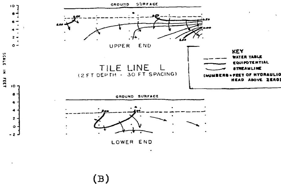
Fig. 4. Flow patterns for tile line L, showing (a) deep seepage on January 16, 1952, and (b) fairly static conditions on May 3, 1951 when evaporation and transpiration also affect the water table.
