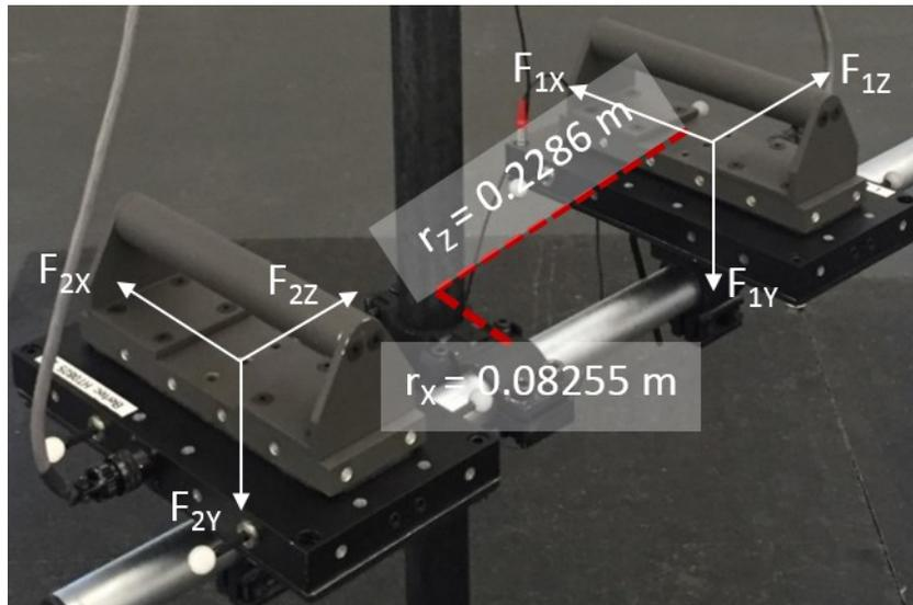
Figure 4 – Vectors used for calculation of net torque in wheelchair turning
