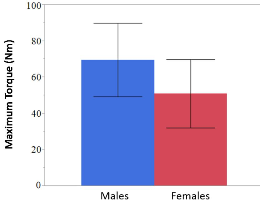
Figure 9 – Max torque produced during wheelchair turning
