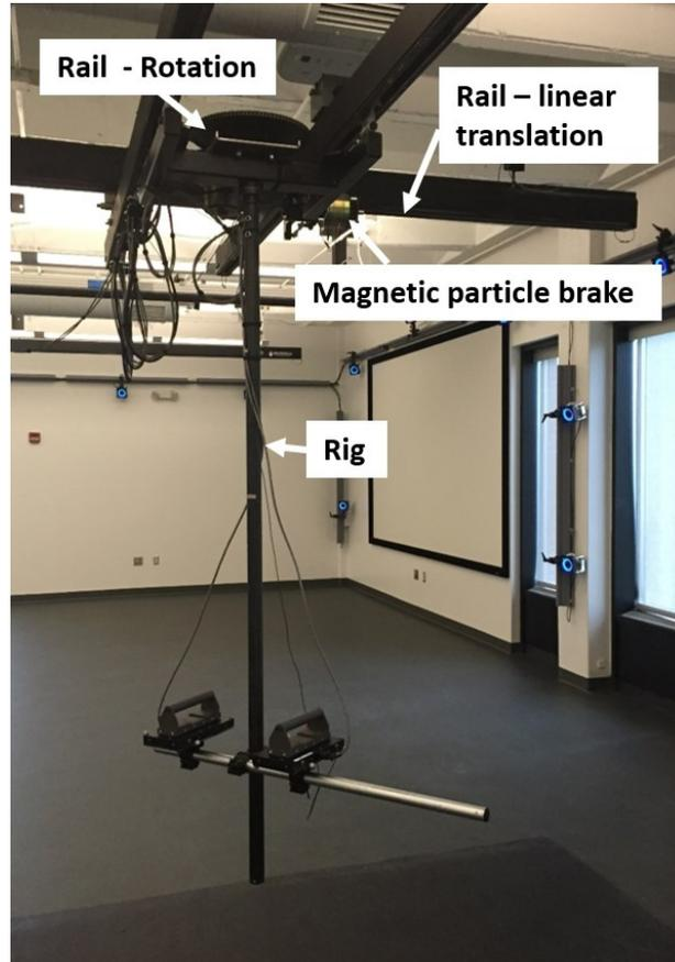
Figure 1 – Overhead braking system and magnetic particle brakes
