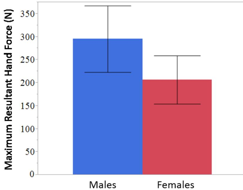
Figure 8 – Max resultant hand forces produced in straight wheelchair pushing
