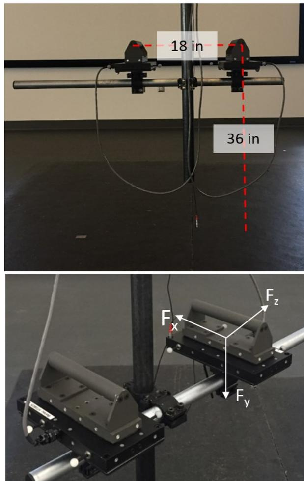
Figure 2 – Experimental setup of hand transducers
