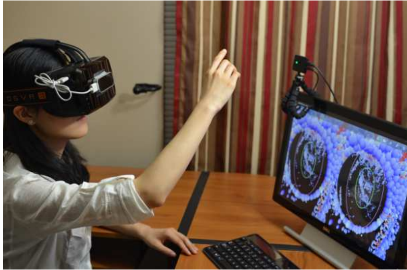
Figure 4.8: The user views stereoscopic glyph visualization in virtual reality headset and controls the GlyphLens by the motion camera mounted on the headset. Head tracking through the camera attached on the monitor is used to change the camera position.
