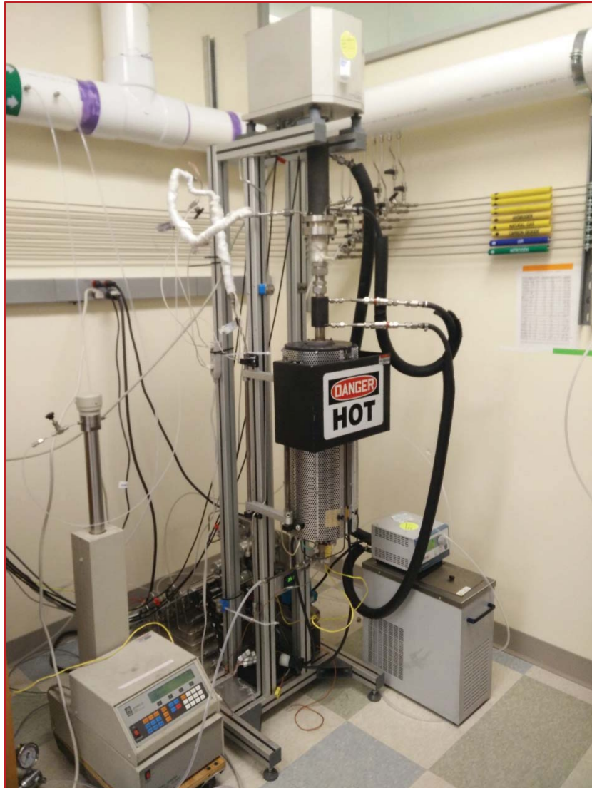
Figure 2.2 TGA setup in the laboratory
