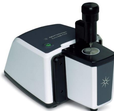
Figure 2.9. Agilent Cary 630 FTIR equipped with diamond ATR sampling accessory. Adapted from (Agilent Technologies, 2013)
