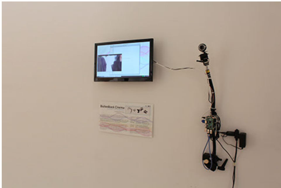
Figure 2: Gallery view of my brain-to-camera interface Biofeedback Cinema . A tool I developed that maps cognitive focus, (observed as alpha waves), to camera focus.
