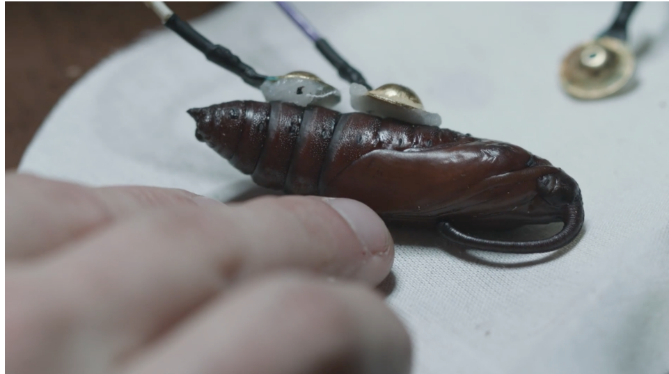
Figure 3: Manduca Sexta moth pupa connected to Open BCI via metal electrodes. 14
