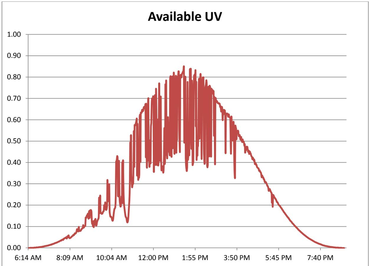
Figure 3. This figure is a representative graph that shows the amount of available ultra-violet light during a typical day as measured by Kipp and Zonen UVS-B-T UV radiometer. The many oscillations are due to cloud cover. The cloud cover can be variable throughout the day. This validates the performance of the ultra-violet badges and demonstrates that the oscillations are due to available ultra-violet light and not badge malfunctions.
