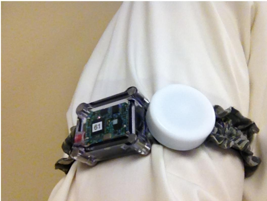
Figure 6. Picture of Daysimeter on left and UVB badge on right.
