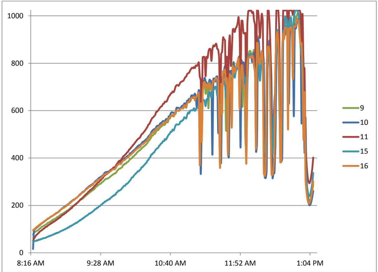
Figure 2. This figure represents the calibration of the ultra-violet badge numbers that were used in the study. The maximum amount of counts the badge will register is 1025. Badges may reach the maximum amount of counts due to the gain control on the badges. To calculate the actual amount of ultra-violet light present, the badge counts were converted using a third order polynomial calibration equation. Consistency among badges is seen even through oscillations due to cloud cover.
