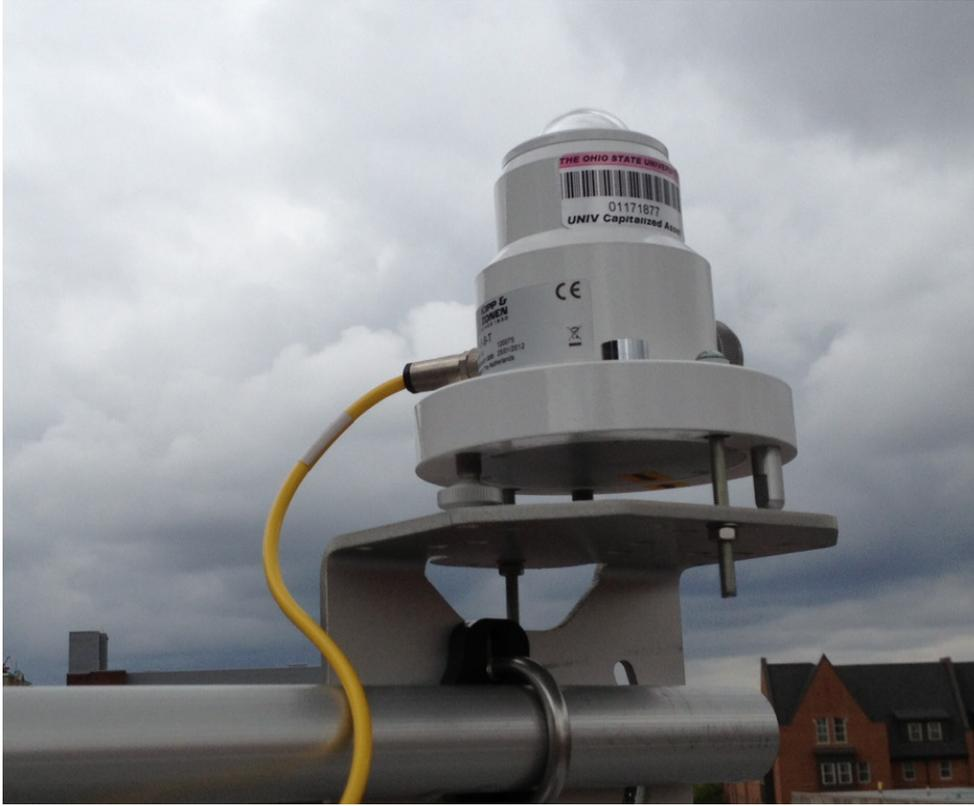
Figure 4. Picture of Kipp and Zonen UVS-B-T UV radiometer.
