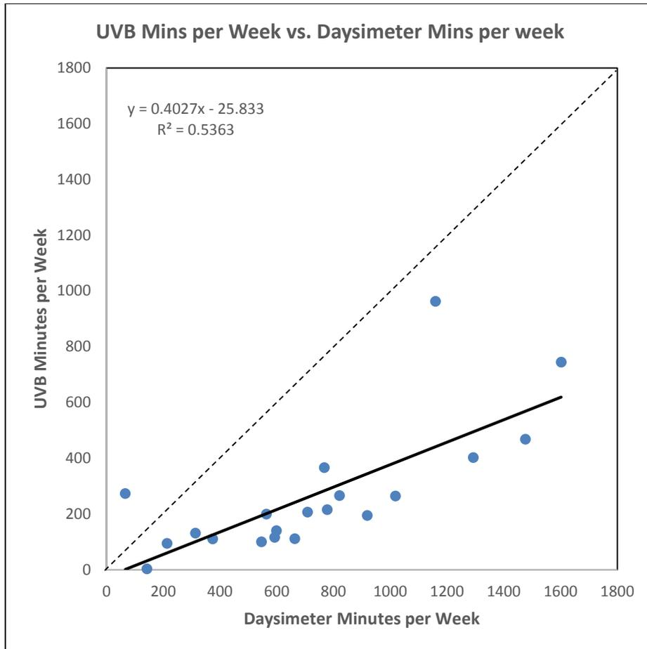
Figure 14. Measurement of minutes per week spent outdoors UVB vs. Daysimeter (the dotted line represents a 1:1 line).
