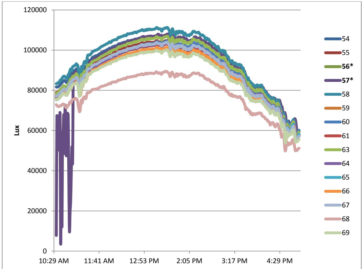
Figure 5. This figure represents the data used to select the Daysimeter visible light badges. The badges demonstrate excellent inter-badge consistency. Badges that were consistent and fell within the center of the center of the distribution were chosen to distribute to subjects first. Badges 57 and 68 were eliminated from use due to inconsistency compared to other badges.
