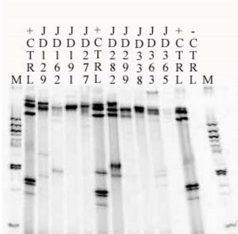
Figure B.3. DGGE gel image of mixed culture 16S rDNA region V3 PCR products. M = 100 bp DNA ladder. + CTRL = mixture of 16S rDNA region V3 PCR products from E. coli , P. strain ADP , K. pneumoniae strain 99, and A. aurescens TCI. CTRL = PCR reaction without template DNA. All other lane designations correspond to the mixed culture serial numbers in Table B.3.
