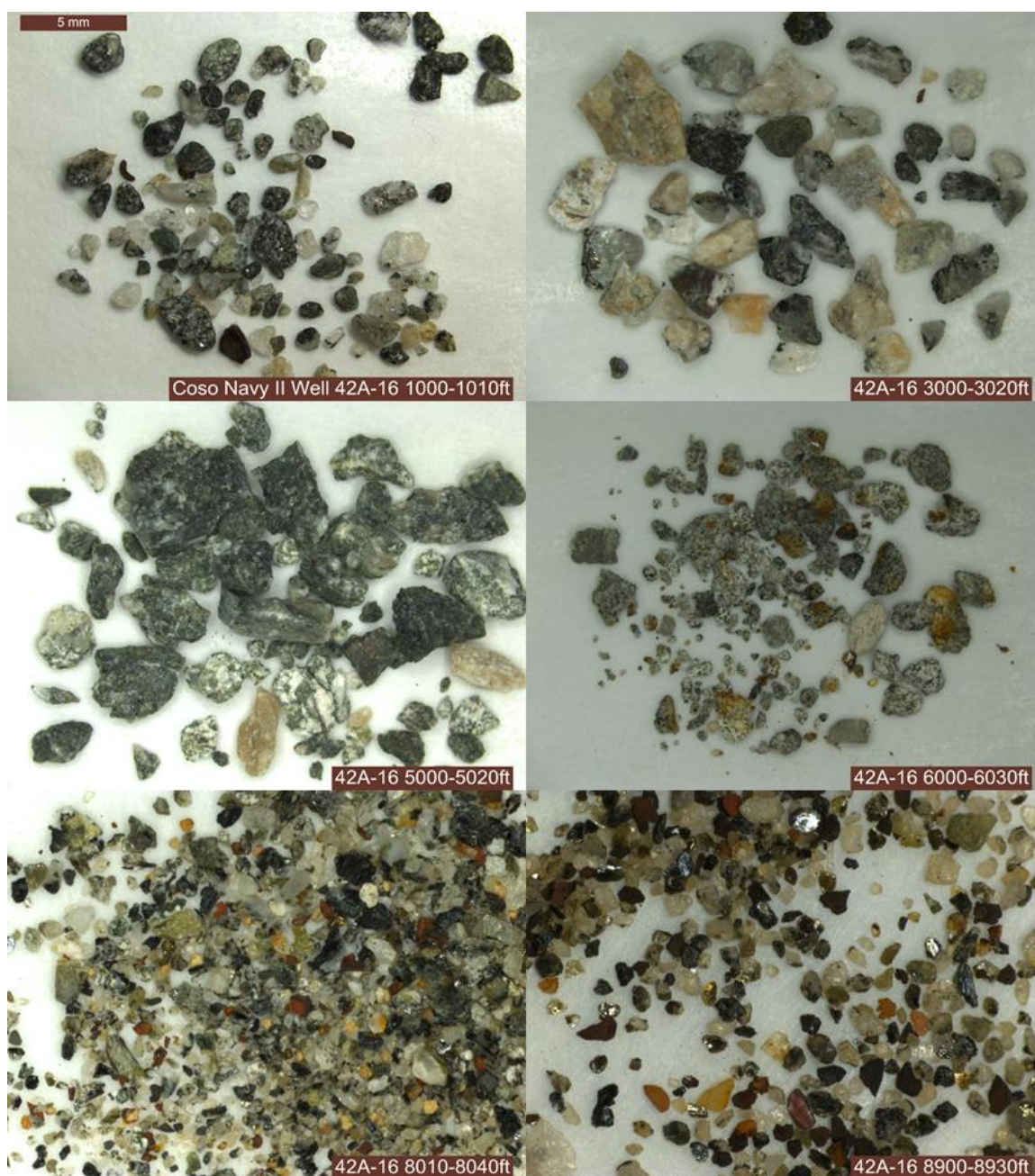
Figure 11. Light microscope images of well cutting samples from Navy II well 42A-16, illustrating some trends of mineralogy with depth. Grains identified include black biotite, dark-gray hornblende, off-white plagioclase, and translucent gray quartz. Chloritization is present (5000-5020 ft), as well as yellow iron oxide staining (6000-6030 ft), and multiple alteration is identified at deeper depth range.
