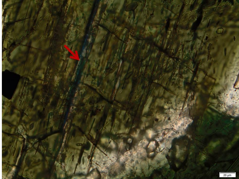
Figure 36. PPL image from Navy II well 42A-16 (8900-8930 ft) shows a long fracture in an amphibole grain. The width is approximately 1-2 \mu\text{m} . The blue proxy is shown inside of the fracture (red arrow). Field of view is 0.3 mm
