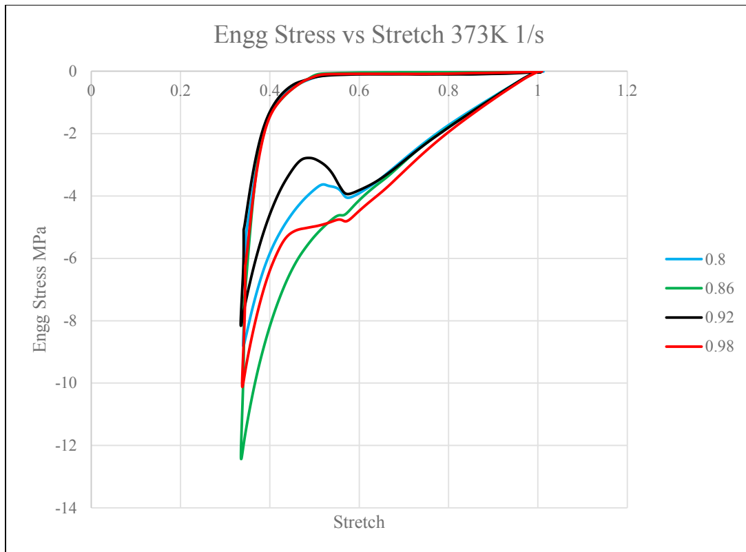
Figure 2.10 Comparison of Stress vs Stretch curves from different samples of same IV at 373K 1/s
