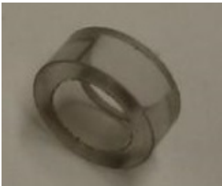
Figure 2.2 Cut preform section used as compression specimen
