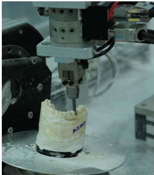
Figure 6: Robot preparing analog space and emergence <sup>xvi</sup>
