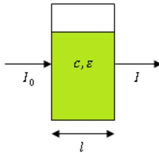
Figure 10: Typical laboratory cuvette used with optical density measurements.
