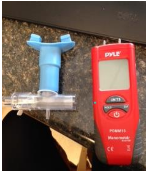
Figure 21. Manometer with flanged mouthpiece used to measure MIP and MEP
