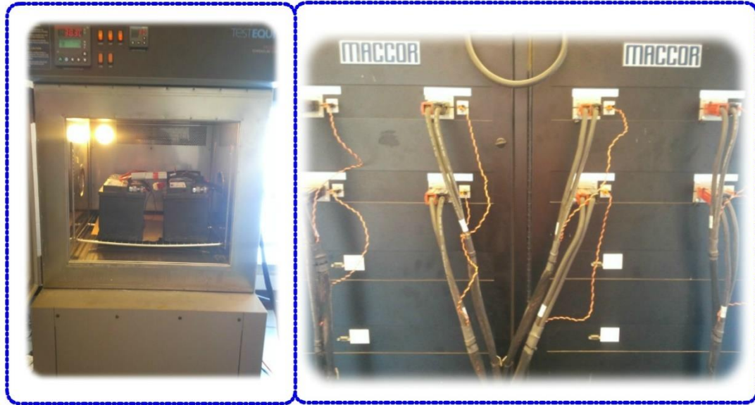
Figure 11: Experimental Setup for Battery Testing (Left: Environmental Chamber with Instrumented Batteries; Right: Maccor Battery Cycler).
