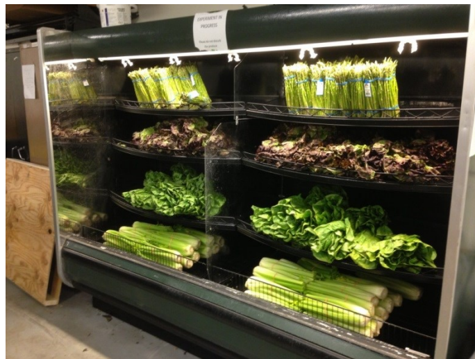
Picture 3.1: Example of the simulation of grocery store rack fresh produce storage a a = celery was not present in this phase of testing, only the top three shelves were used
