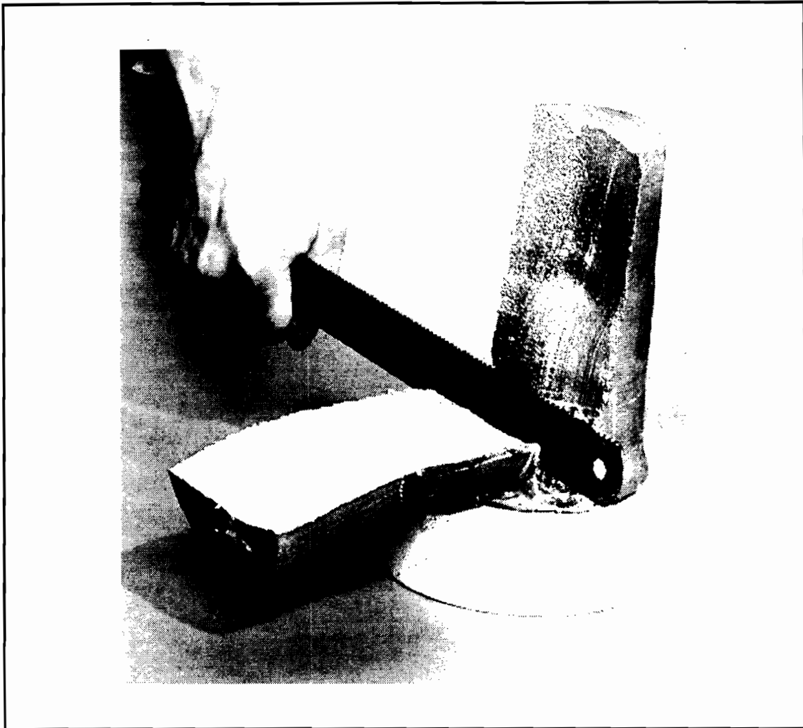
Figure 2.1: A semi-solid material, being cut with a saw blade while standing free [Endabmessungsnahe Fertigung-Ur/Umformtechnik (EFU) brochures, 1994].
