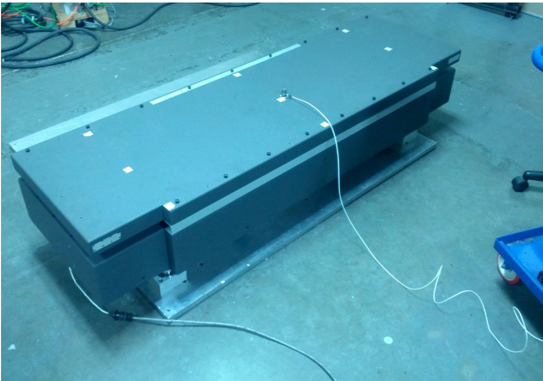
Figure 55: Accelerometer Placement on the Treadmill Force Platform.
