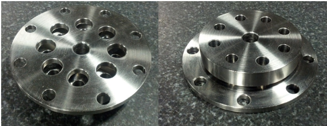
Figure 40: Stainless Steel Spacers for Prototype Pylon Design.
