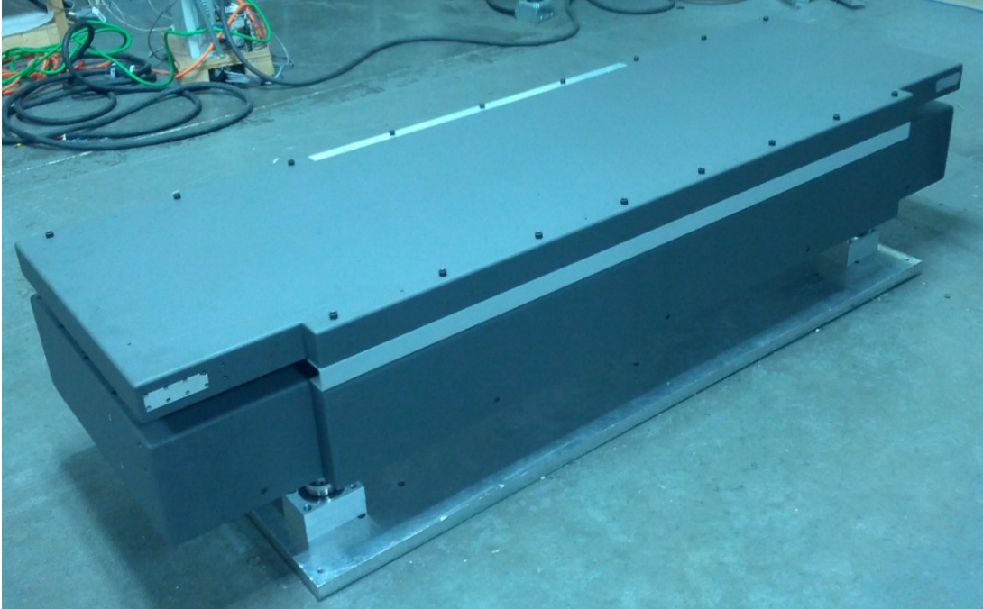
Figure 51: Fully Assembled Treadmill Force Platform with Pylons Mounted.
