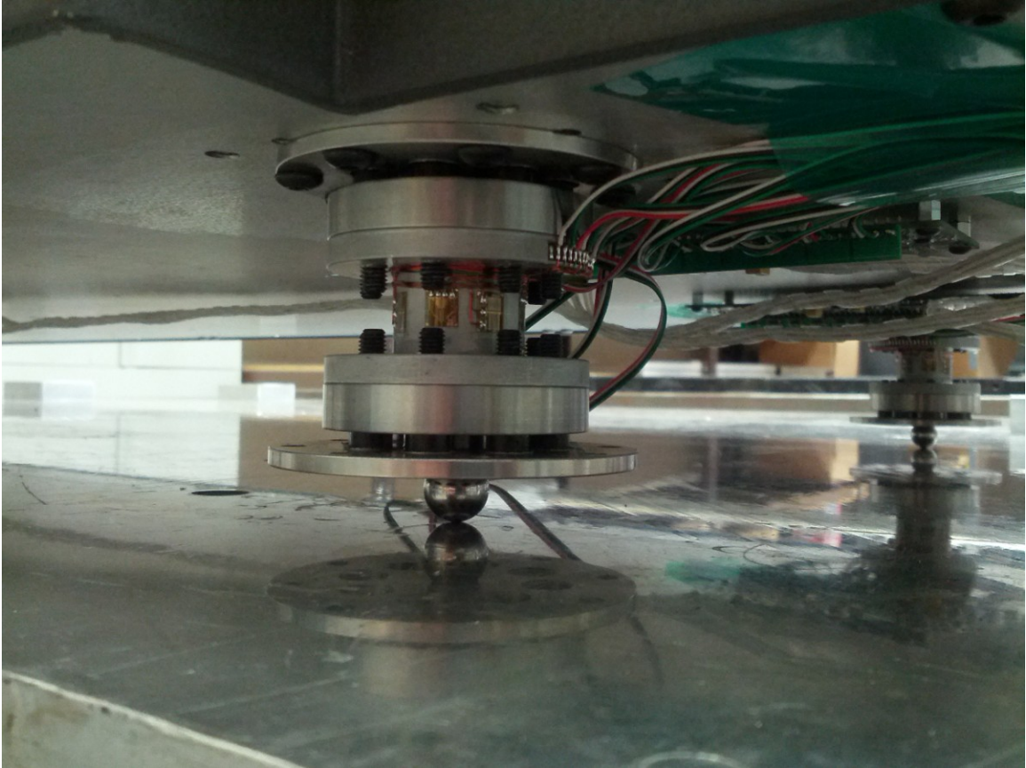
Figure 54: Ball Bearing Setup Used to Test the Second Set of Prototype Pylons.
