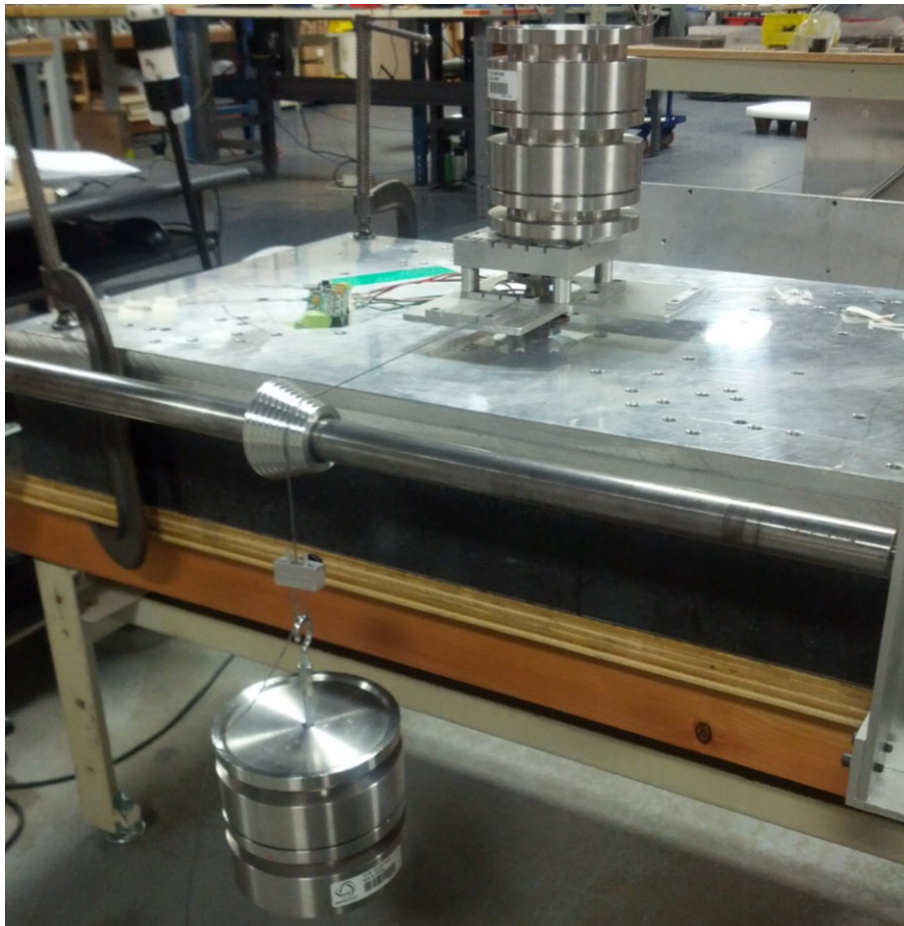
Figure 44: Calibration Plate Setup with Vertical and Shear Calibration Weights Applied.
