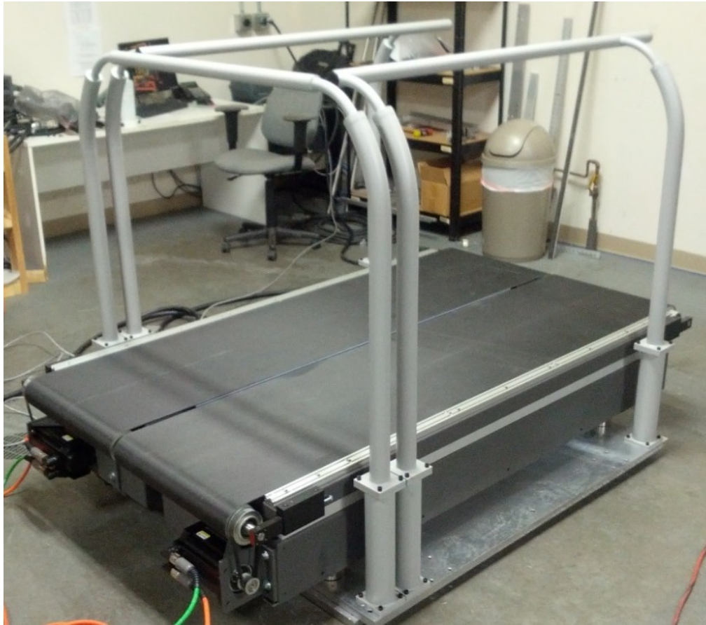
Figure 5: Fully Assembled Dual Belted Bertec Force Measurement Treadmill.
