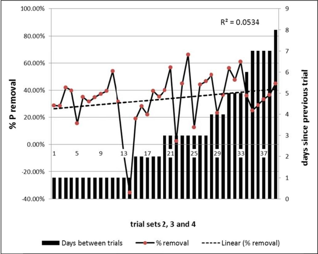
Figure 10: Effect on removal rate of increasing days between trials.
