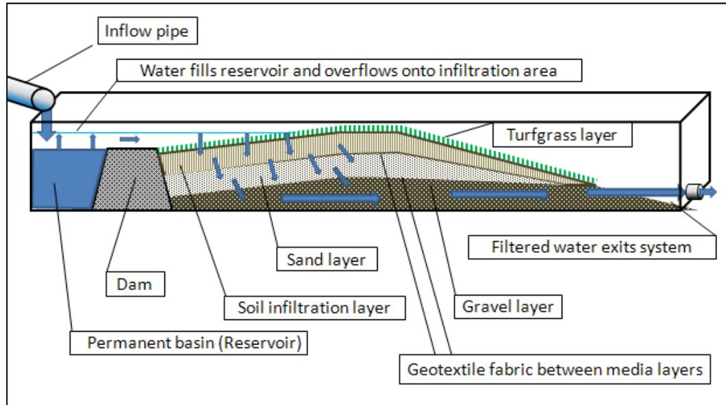
The lab scale filtration basin model was used to perform multiple research trials in which a known amount of artificial storm water with a known concentration of DRP and sediment was applied at a known inflow rate. Nitrate was also evaluated although no removal was expected. Water from the inlet and outlet, and soil and grass samples were analyzed to determine fate and transport of the contaminants.
