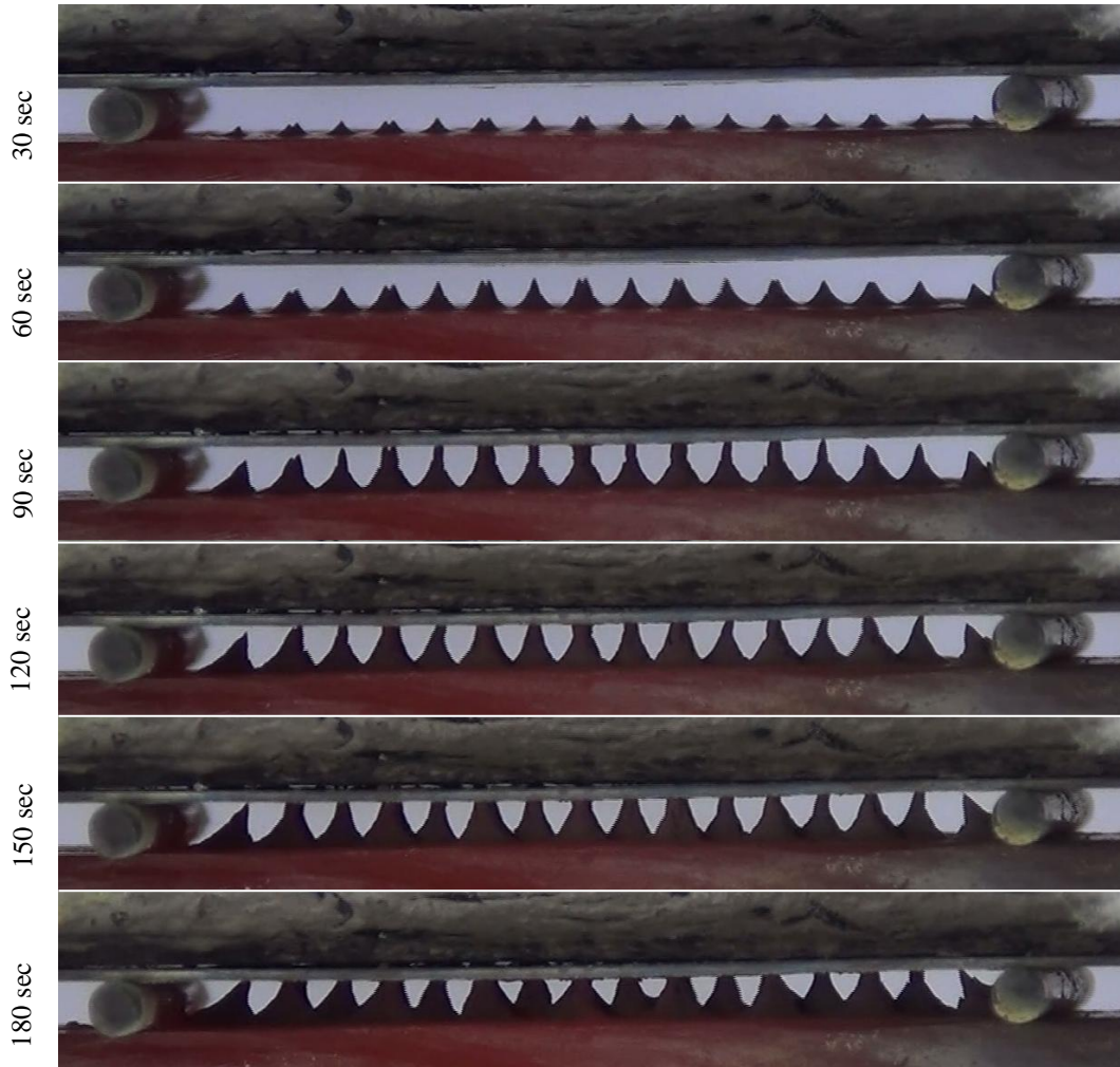
Figure 4.9 – Video frames from test 8 (low flow rate, high temperature, with flame heating) showing cones penetrating impingement holes.
