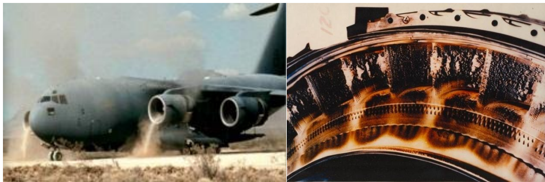
Figure 1.1 – (left) Dust ingestion into C-17 aircraft and (right) volcanic ash deposition on turbine vanes [2]
