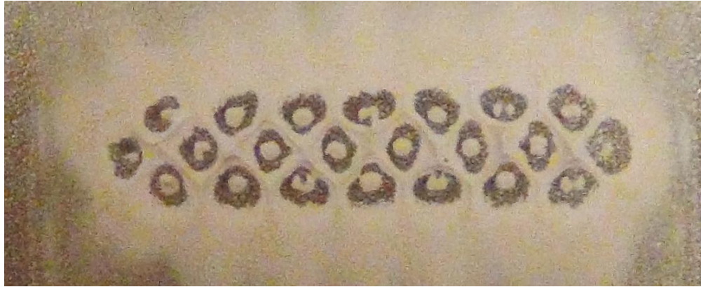
Figure 4.4 – Photograph of post-test impact plate from test 14a at intermediate flow rate and ambient temperature.
