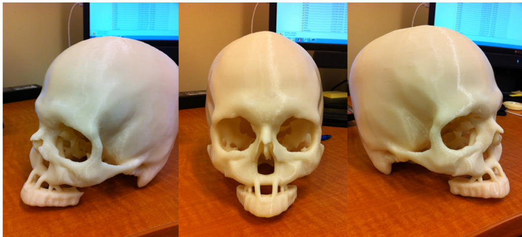
Figure 4.4. Skull model fabricated with fused decomposition modeling
