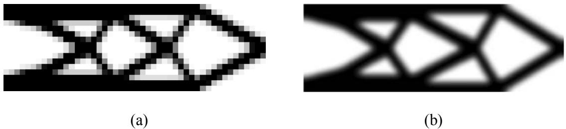
Figure 2.10. 2D cantilever beam solutions (mesh size: 48 \times 12 ): (a) element based topology optimization (Q4) (b) Multiresolution topology optimization (Q4/n25)
