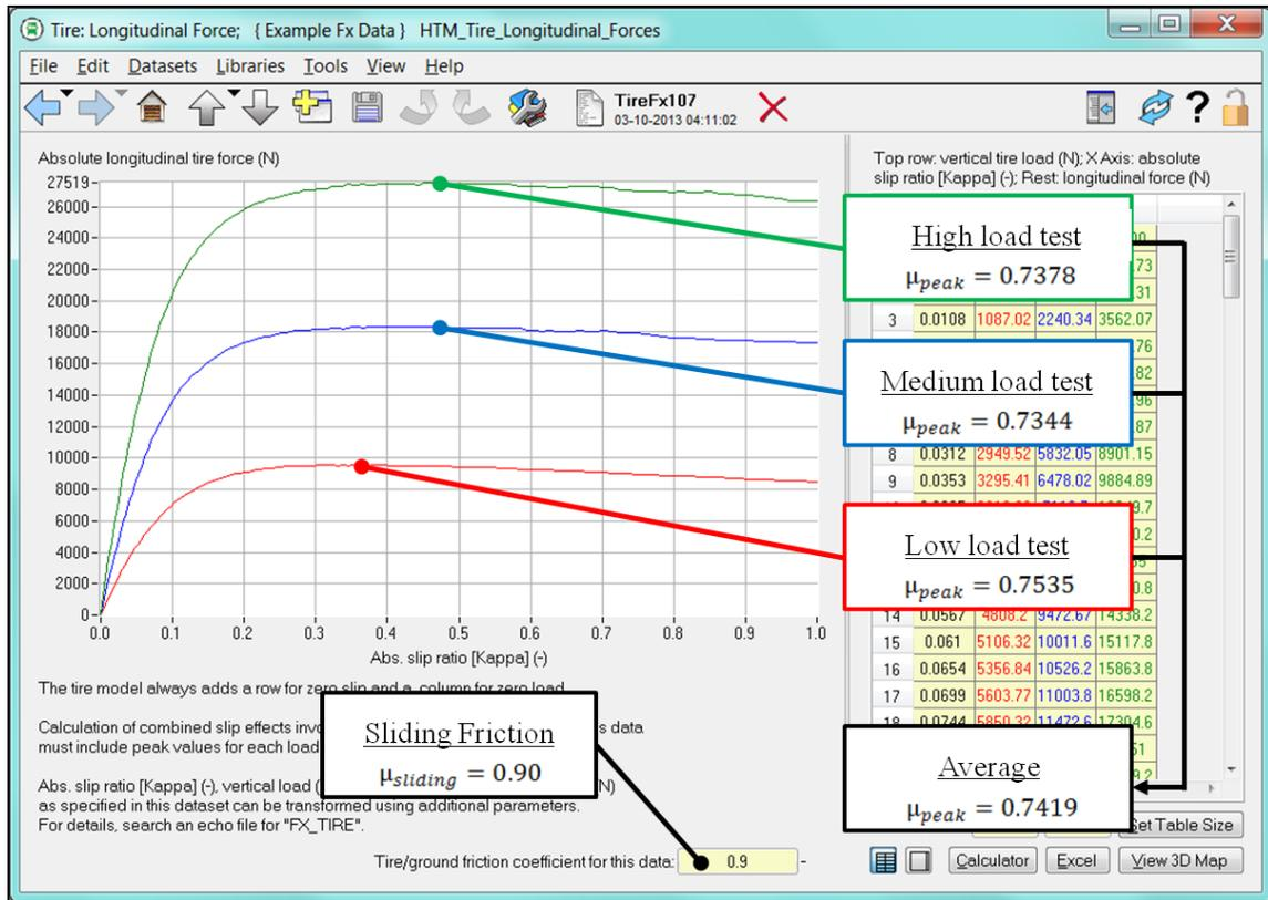
Figure 5.1: TruckSim Tire Efficiency
