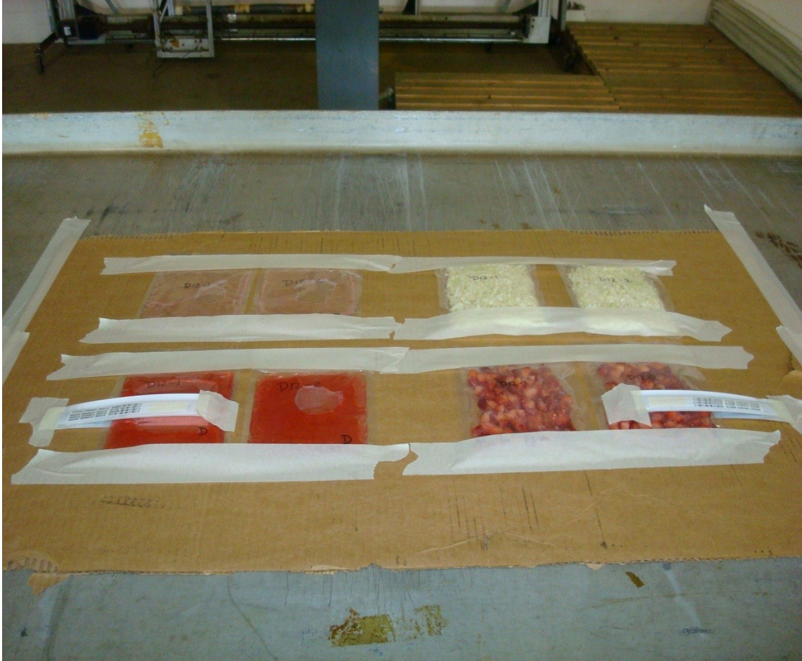
Figure 10. Clockwise from top left, two packages of PBS, cabbage, strawberries, and DMEM were secured on a cardboard sheet to be treated with e-beam. Cardboard sheets were secured to the cart conveyor system. Alanine dosimeters were secured to the top and bottom of the packages (bottom row).
