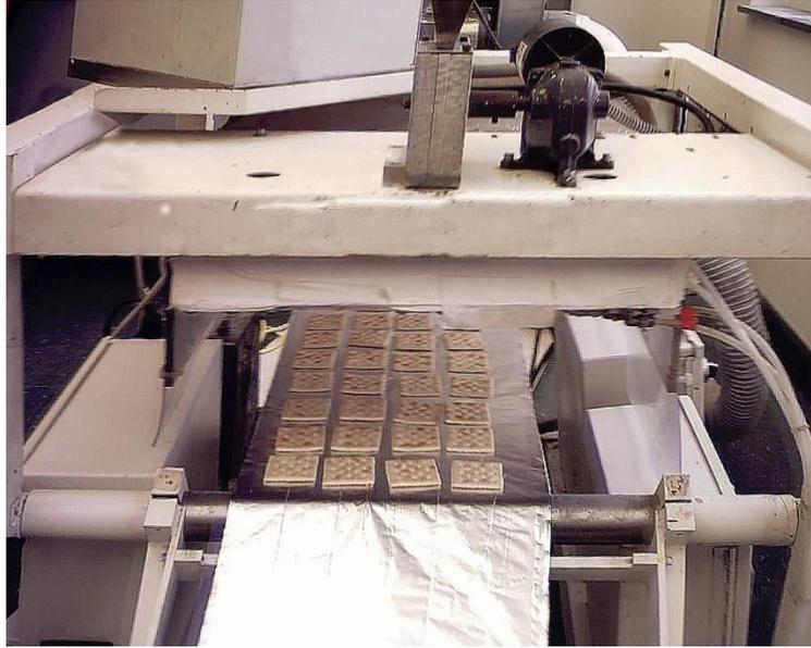
**Figure 2.** Saltine crackers being coated in a conveyor belt coating system.
