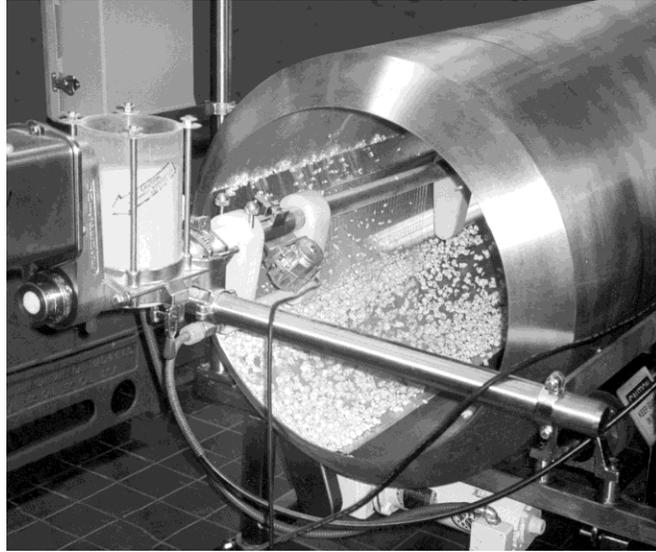
**Figure 1.** A tumble drum coating system used in coating popcorn with salt.
