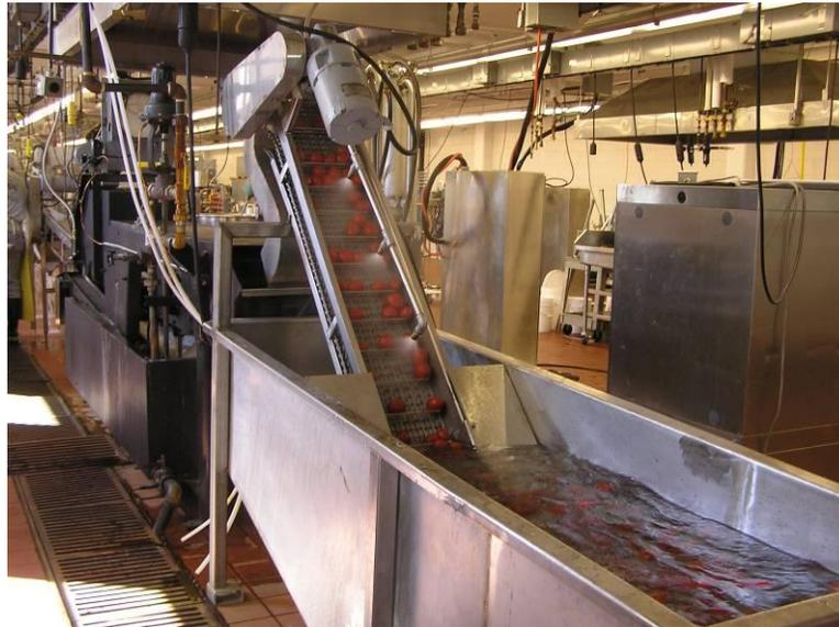
**Figure 8.** Tomato washing in a tank before transporting to the lye peeler.
