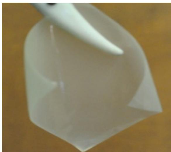
Figure 4.29 A picture of sulfuric acid modified chitosan membrane.
