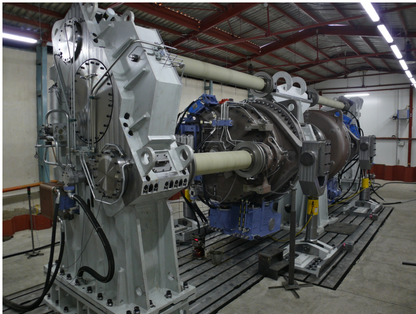
Figure 4.16: FC5500 back-to-back, power circulating experimental test rig configuration [48].
