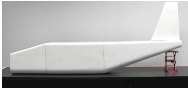
Figure 7.19: Three regions of simplified Dakota UAV fuselage with the vertical stabilizer.
