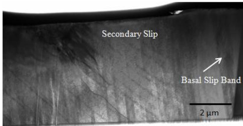
Figure 1.10: STEM image of foil from sample with a total strain over 25%. Zone axis:  $\langle 1\bar{1}01 \rangle$ ;  $\mathbf{g}_{\langle 011 \rangle}$
