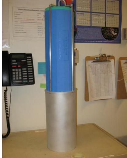
Figure 28: Low Temperature system for the neutron experiment.
