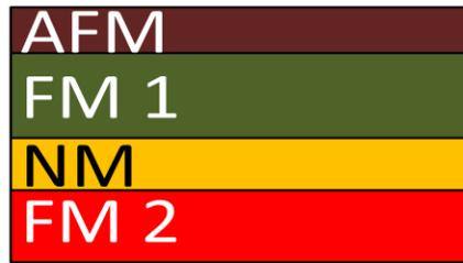
Figure 3: Spin valve device
