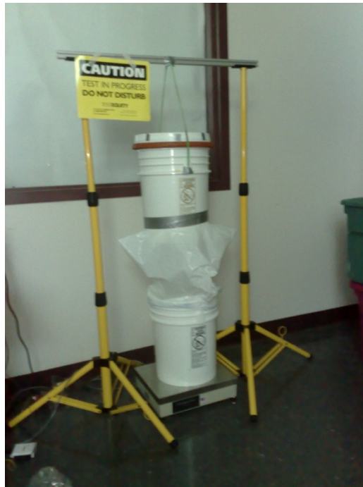
Figure 3.1: Model experimental setup for flow experiments conducted for different filter variants.
