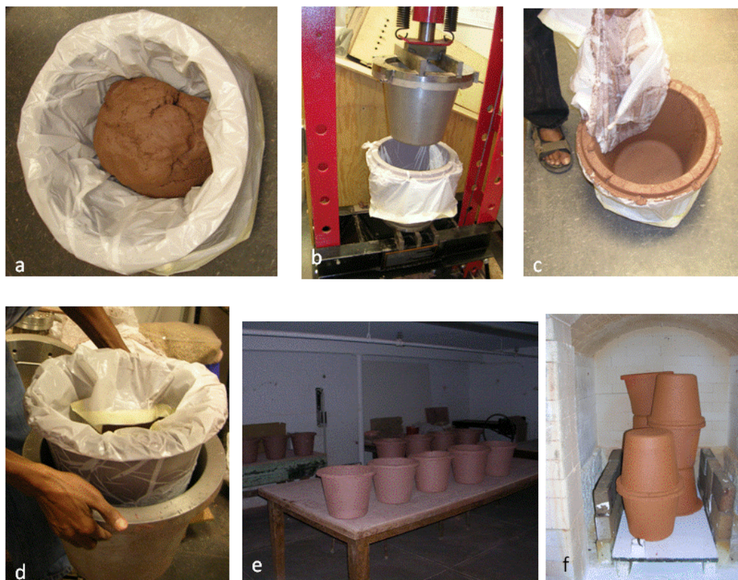
Figure 2.1: Step by step manufacturing of ceramic filter from moistened balls of clay and sawdust blend.
