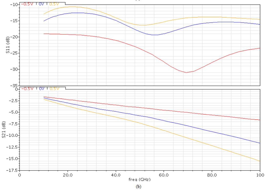
Figure 4.9 S-parameter simulation result (a) W-band (b) V-band
