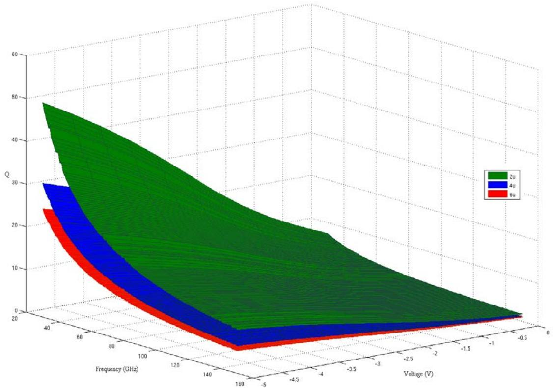
Figure 3.5 Quality factor performance vs. frequency and reverse bias voltage for varying anode length
