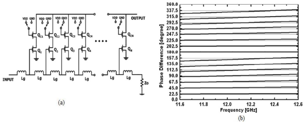
Figure 2.5 (a) Proposed topology (b) Measured 4-bit phase shift in steps of  $22.5^\circ$  [5]
