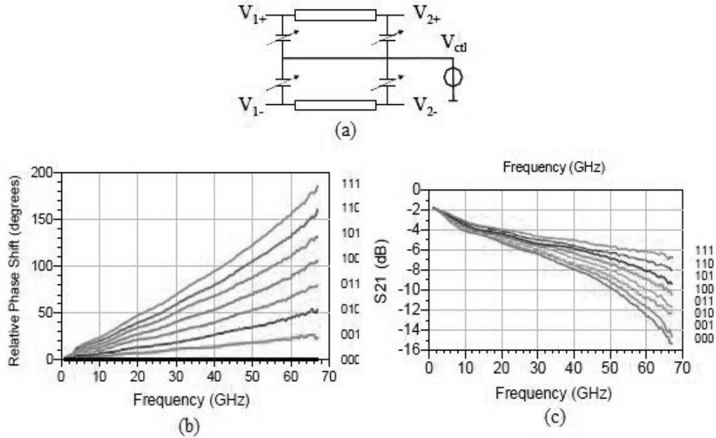
Figure 2.6 (a) Proposed differential phase shifter loaded with differential varactors (b) Relative phase shift for 8 different states (c) Corresponding insertion loss [6]
