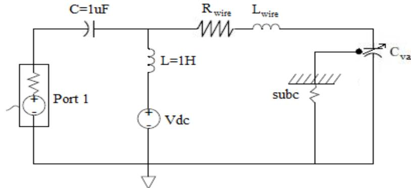
Figure 3.3 One-port simulation circuit
