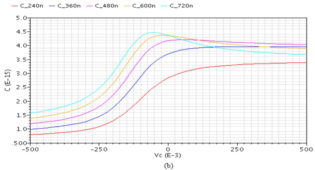
Figure 3.10 Capacitance vs. (a) width (b) length at 100 GHz
