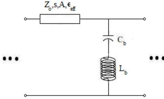
Figure 2.3 Line cell model, where  $Z_o$  is unloaded line impedance,  $s$  is the periodic spacing of bridge,  $A$  is unloaded line attenuation,  $\epsilon_{eff}$  is effective dielectric constant,  $C_b$  is bridge capacitance and  $L_b$  is bridge inductance [2]
