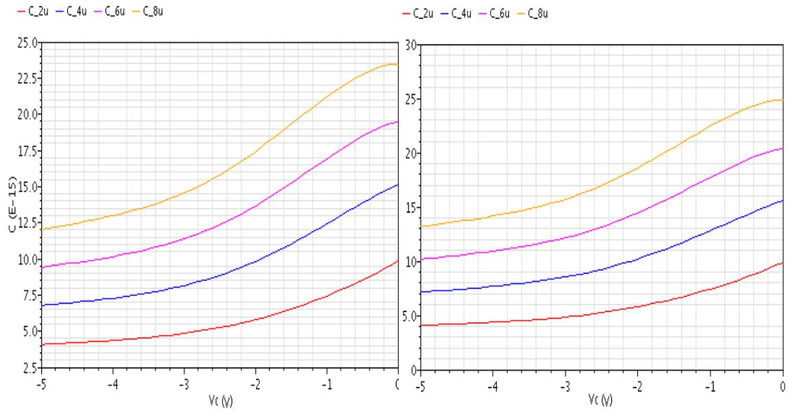
Figure 3.6 capacitance vs. (a) anode length (b) anode width at 100 GHz
