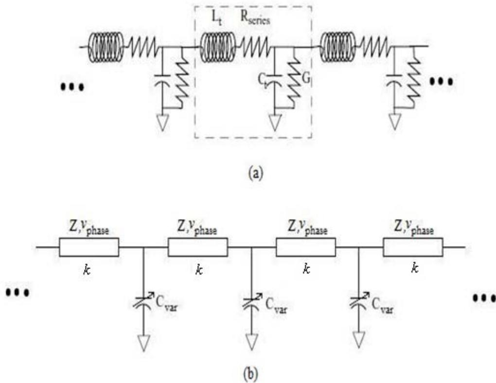
Figure 2.1(a) Distributed transmission line model (b) Loaded transmission line
