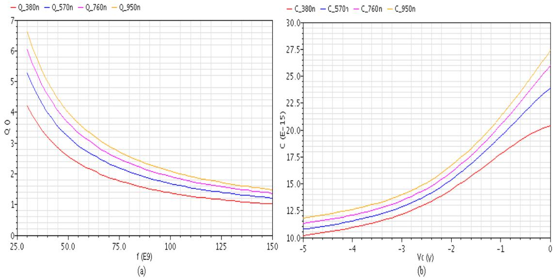
Figure 3.7 (a) quality factor vs. frequency (b) capacitance vs. reverse bias voltage, for different cathode widths
