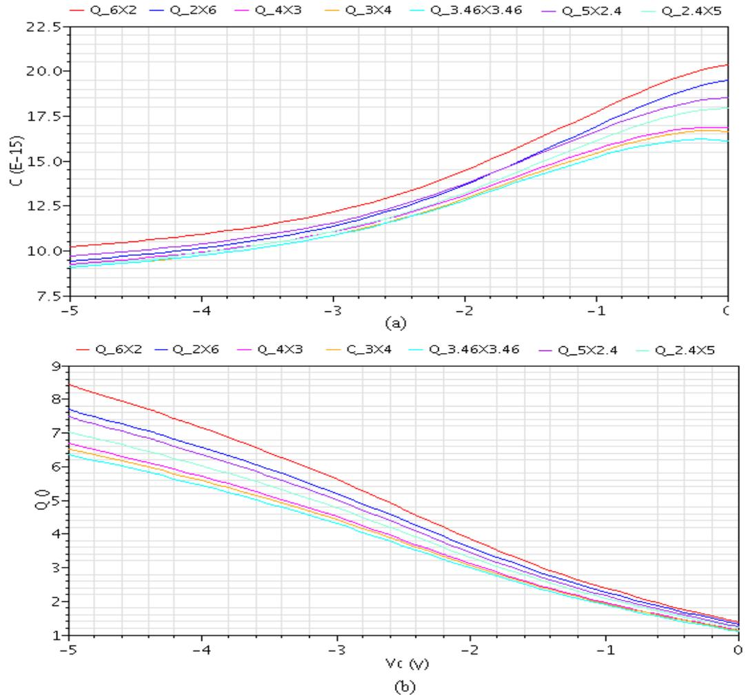
Figure 3.4 (a) capacitance (b) quality factor vs. junction area at 100 GHz
