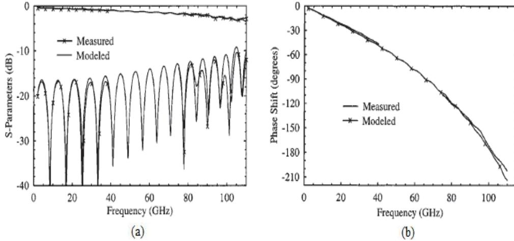
Figure 2.4 (a) S-parameter at maximum bias of 26V (b) Phase shift at maximum bias (26V) [3]
