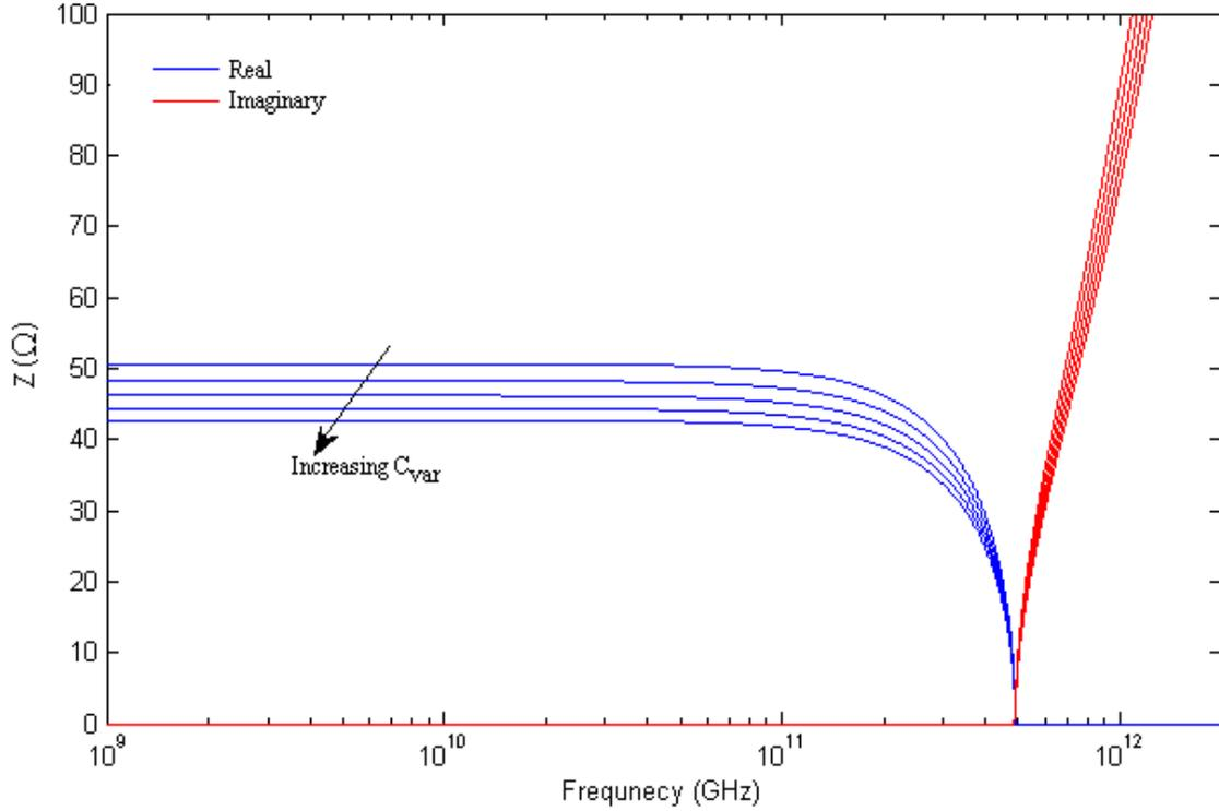
Figure 2.2 Effect of Bragg frequency on line characteristic impedance
