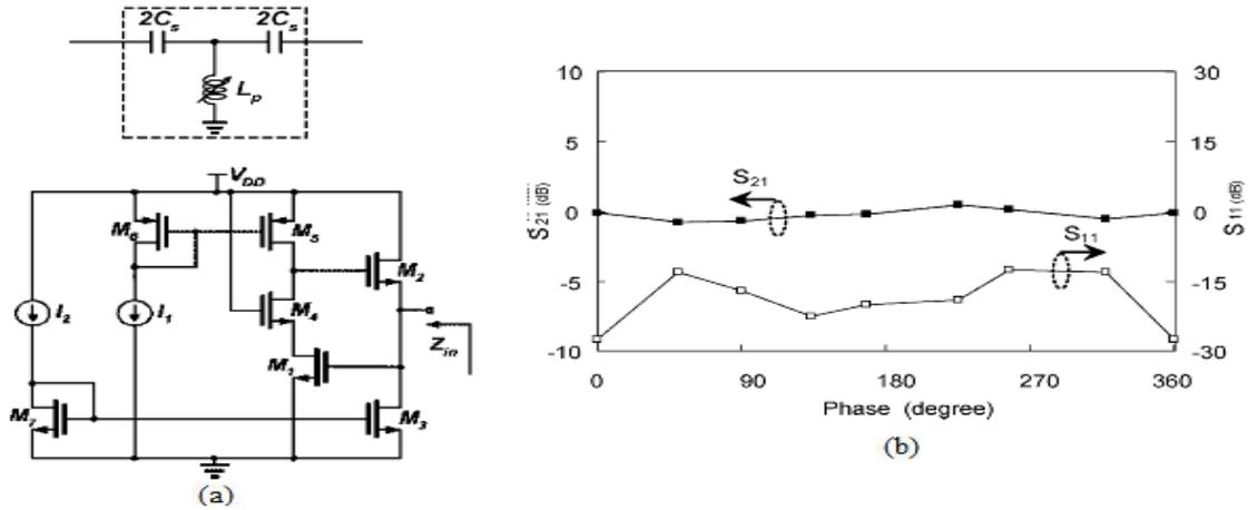
Figure 2.7 (a) Proposed line with tunable inductance with schematic (b) Measured S-parameters at 4GHz [7]
