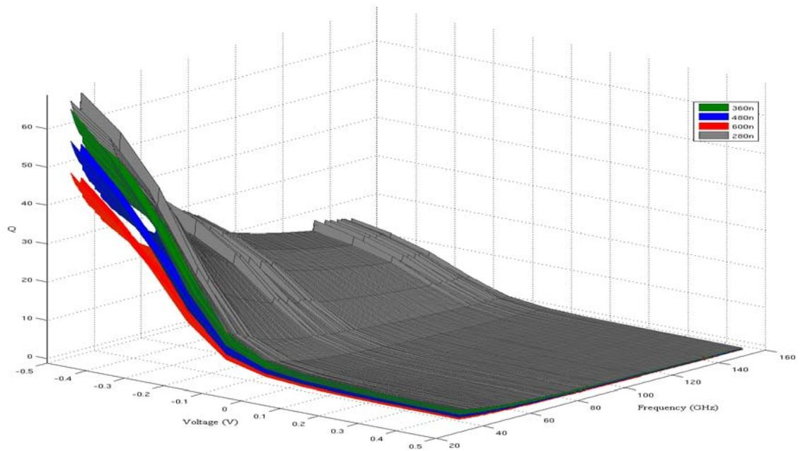
Figure 3.9 Quality factor performance vs. frequency and voltage for varying length
