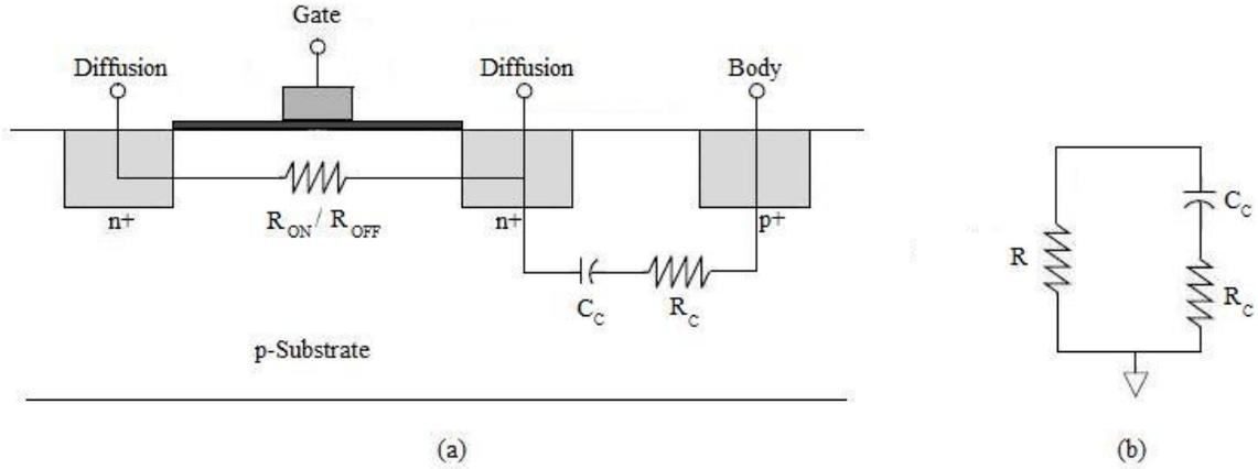
Figure 4.4 (a) NMOS switch cross section (b) Equivalent switch resistance model
