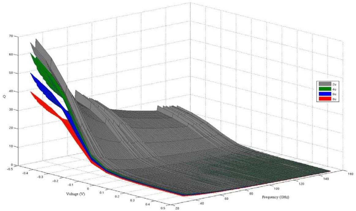
Figure 3.8 Quality factor performance vs. frequency and voltage for varying width
