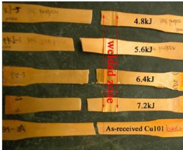
Figure 6.4 Fracture of lap shearing tests.
