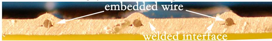
(c) Welded sample for aluminum plate with steel wire embedded
