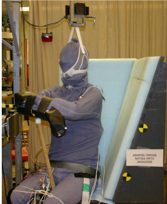
Figure 2.9: Pre-test Positioning of Oblique Impact
