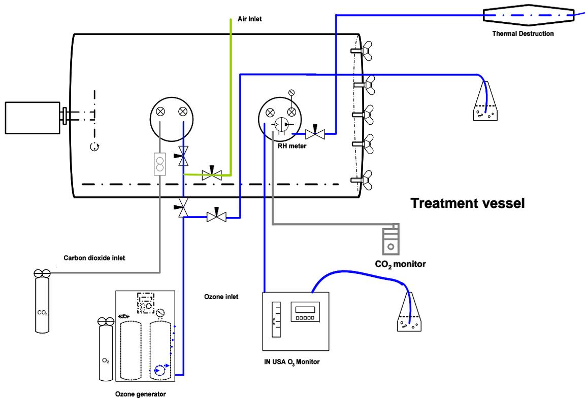
Figure 4.1 Schematics of the gaseous treatment system for fresh strawberries.
