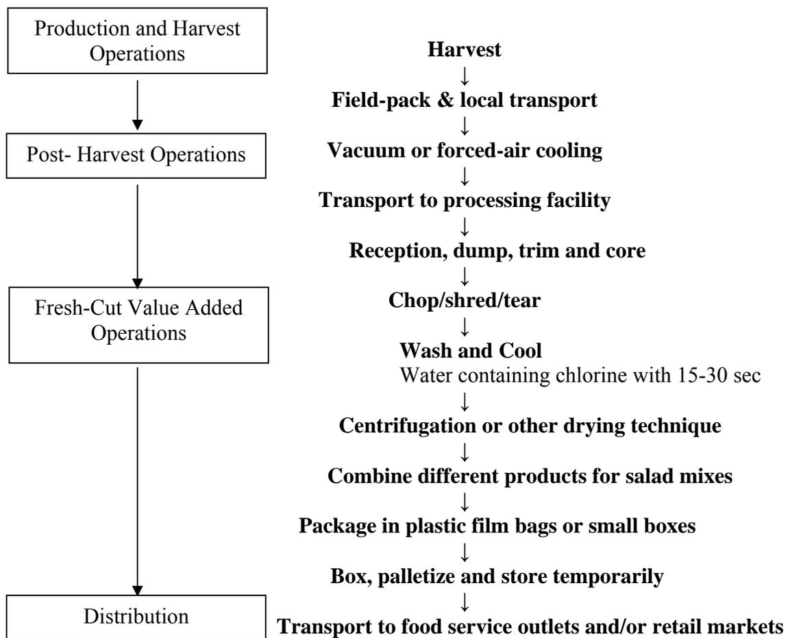
Figure 1.8. Preparation of minimally processed fresh-cut leafy greens (Adapted from Kader, 2002).
