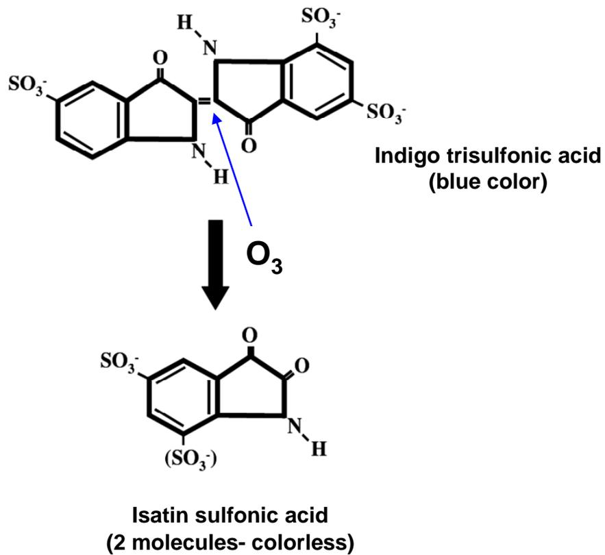
Figure 1.5. Reaction between ozone and indigo trisulfonic acid (Modified from Bader and Hoigné, 1981).
