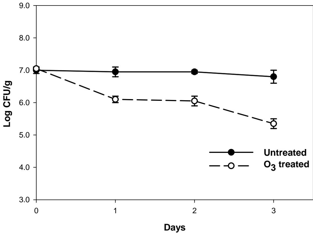
Figure 3.4. Changes in population of *Escherichia coli* O157:H7 on fresh spinach when the inoculated produce treated with continuous ozone at 16 mg/kg (10 ppm; vol/vol) in refrigerator ( $2\pm 1^{\circ}\text{C}$ ) for up to 3 days (SanTrans process). Data shown are averages of three independent trials. Error bars represent  $\pm$  standard error.
