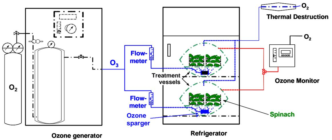
Figure 3.1. Equipment used for treating fresh produce with low levels of ozone during refrigerated storage, mimicking fresh produce transportation (SanTrans process).
