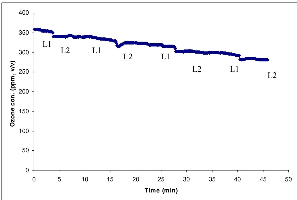
Figure 2.5. Ozone concentration measured at different location inside the treatment vessel. L1 represents a sampling point close to the periphery of the vessel, while L2 represents a sampling point close to the product.
