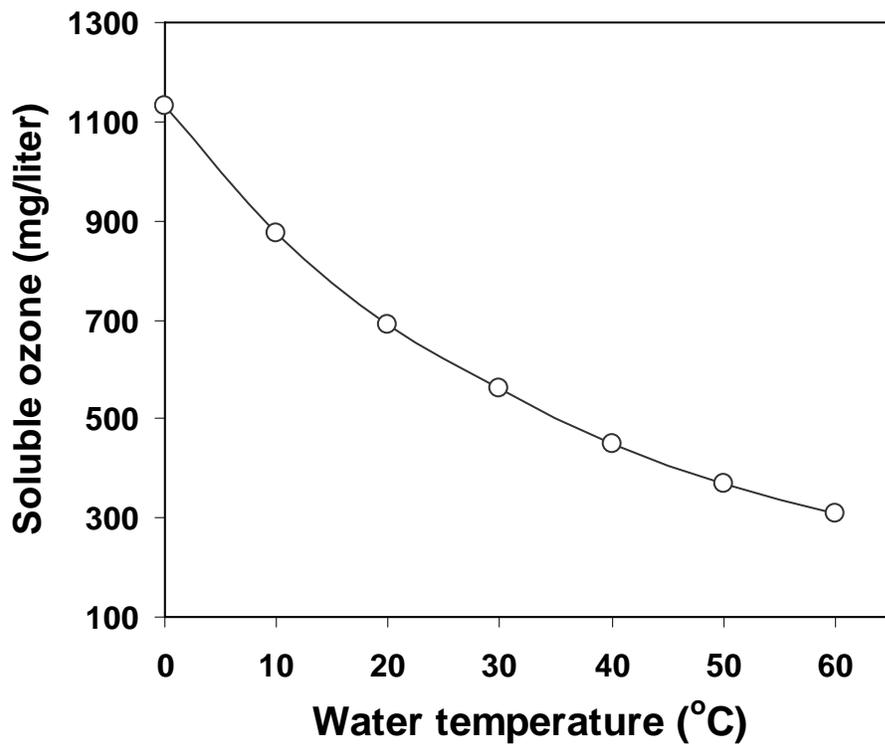
Figure 1.2. Solubility of gaseous ozone in water at atmospheric pressure (101.3 kPa) and different temperatures (Horváth et al., 1985).
