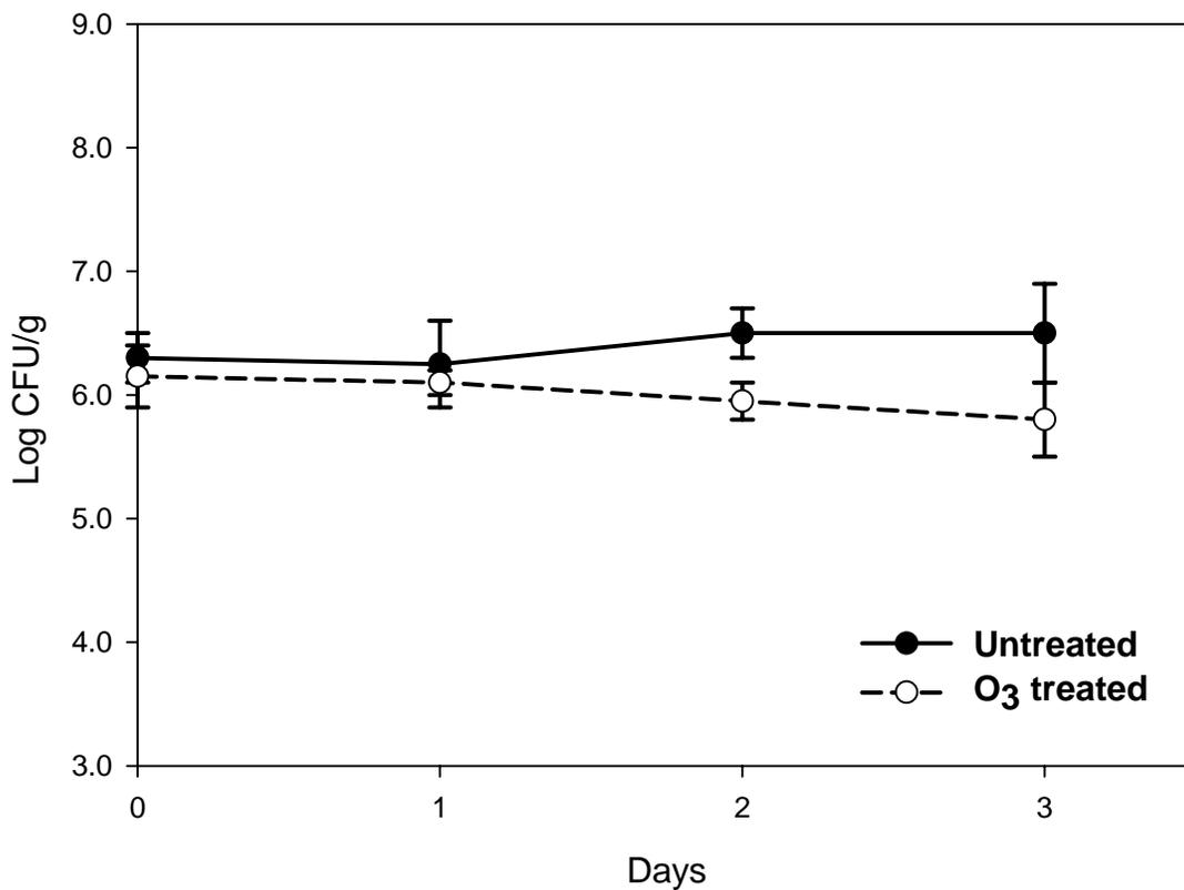
Figure 3.3. Changes in natural microbiota of baby spinach when the produce treated with continuous ozone at 8 mg/kg (5 ppm; vol/vol) in refrigerator ( $2\pm 1^{\circ}\text{C}$ ) for up to 3 days. Data shown are averages of two independent trials. Error bars represent  $\pm$  standard error.
