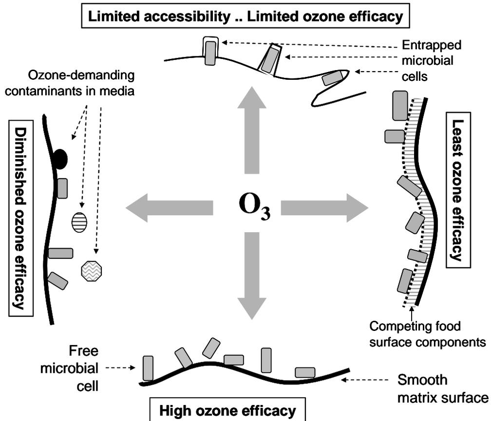
Figure 1.6. Schematic representation of accessibility of ozone to target microorganisms as related to the efficacy of the sanitizer.
