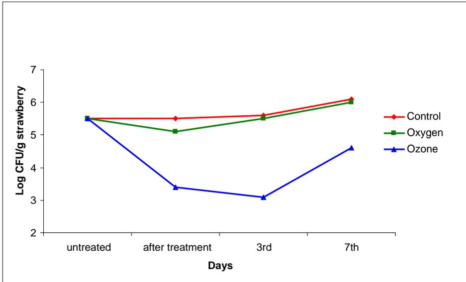
Figure C.14. Changes in yeast and mold count of strawberries that were treated with ozone (0.4 g/kg) or oxygen for 24 h and stored for 7 days at 20 °C and 95-100% RH.
