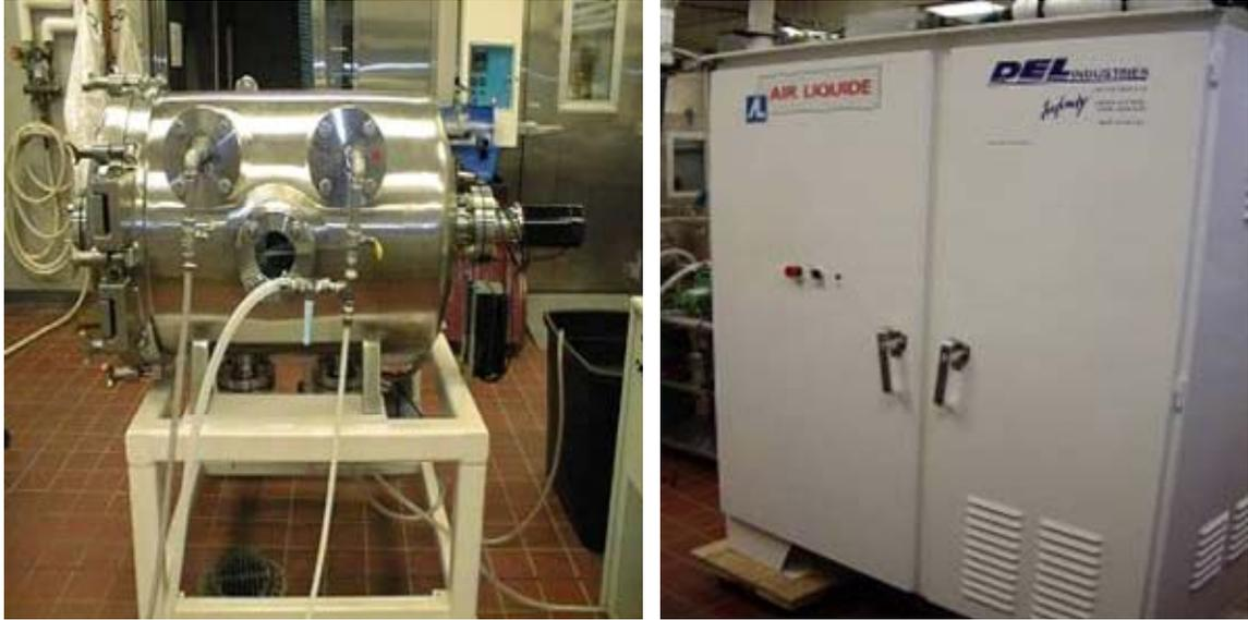
Figure C.4. Experimental setup 2 to treat fruits with gaseous ozone under pressure
