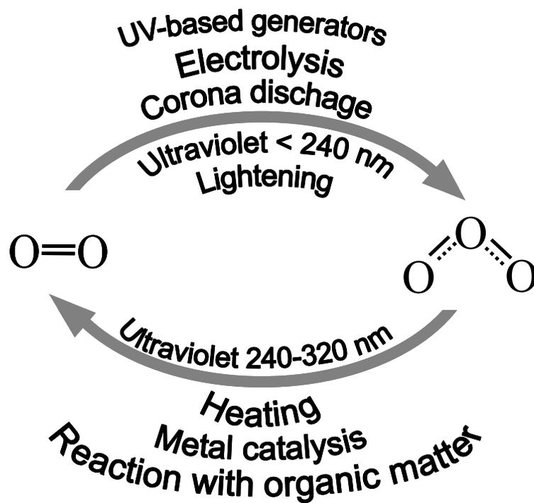
Figure 1.1. Formation and decomposition of ozone in nature or through industrial processes. [ $O_2$ : oxygen;  $O_3$ : ozone; inner reactions: occur in nature; outer reactions: industrially generated]
