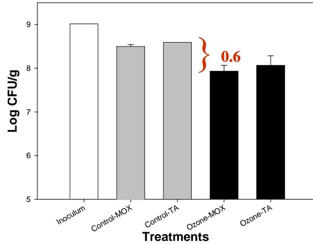
Figure C.5. Changes in population of *L. monocytogenes* OSY-328 on strawberries when treated with 14g/kg (19 g/m<sup>3</sup>) dry ozone at 10 psig for 10 min using Setup 2. *Listeria* populations were enumerated on MOX agar and TA. Values are the average of duplicate samples of two experiments.
