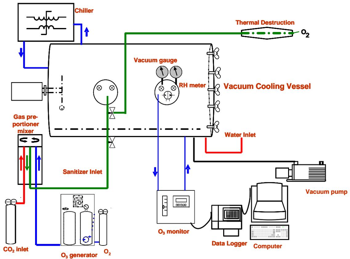
Figure 2.2. Setup used for treating fresh produce with ozone, in tandem with vacuum cooling (SanVac process).
