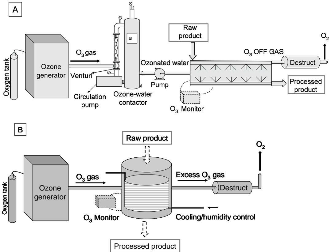
Figure 1.7. Conceptual aqueous and gaseous ozone treatment systems that may be relevant to food applications. [A: aqueous, B, gaseous]
