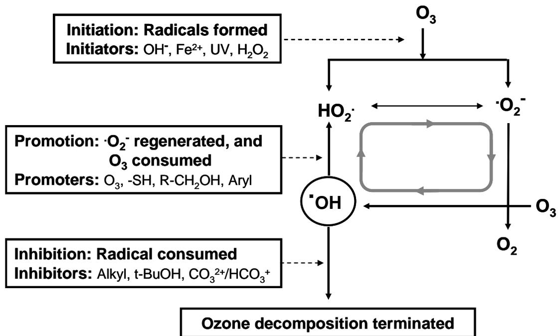
Figure 1.3. Ozone decomposition and free radical formation reactions (Adapted from Khadre et al., 2001). [ $\text{O}_2$ , oxygen;  $\text{O}_3$ , ozone;  $\cdot\text{OH}$ , hydroxyl radical;  $\cdot\text{O}_2^-$ , superoxide anion radical;  $\text{HO}_2\cdot$ , hydroperoxide radical]
