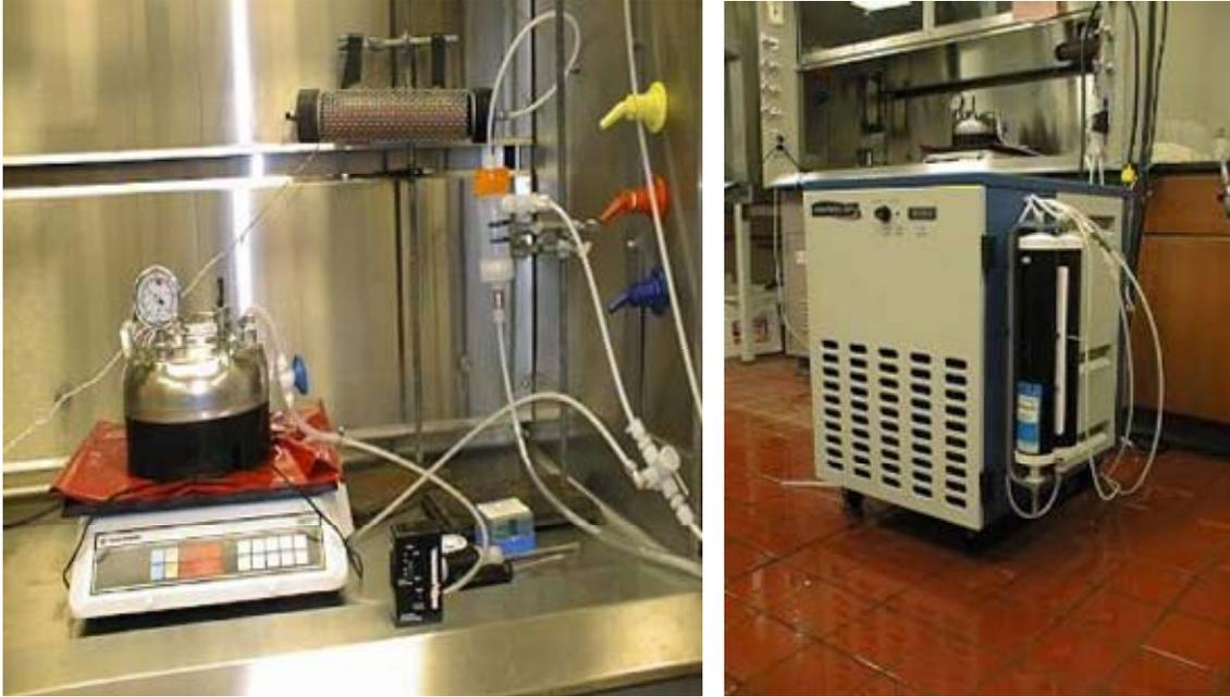
Figure C.1. Experimental setup 1 to treat fruits with gaseous ozone under pressure
