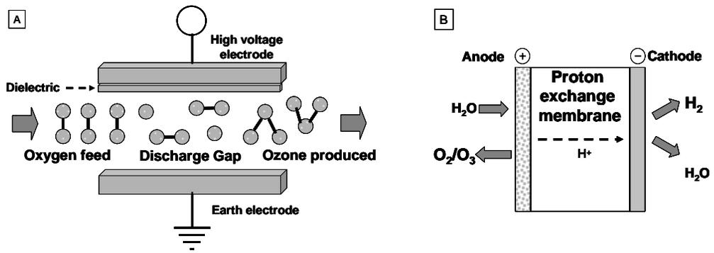
Figure 1.4. Ozone generation by corona discharge method (Adapted from Rice et al., 1981) and electrolysis of water (Lynntech, 1998). [A, corona discharge; B, electrolysis]
