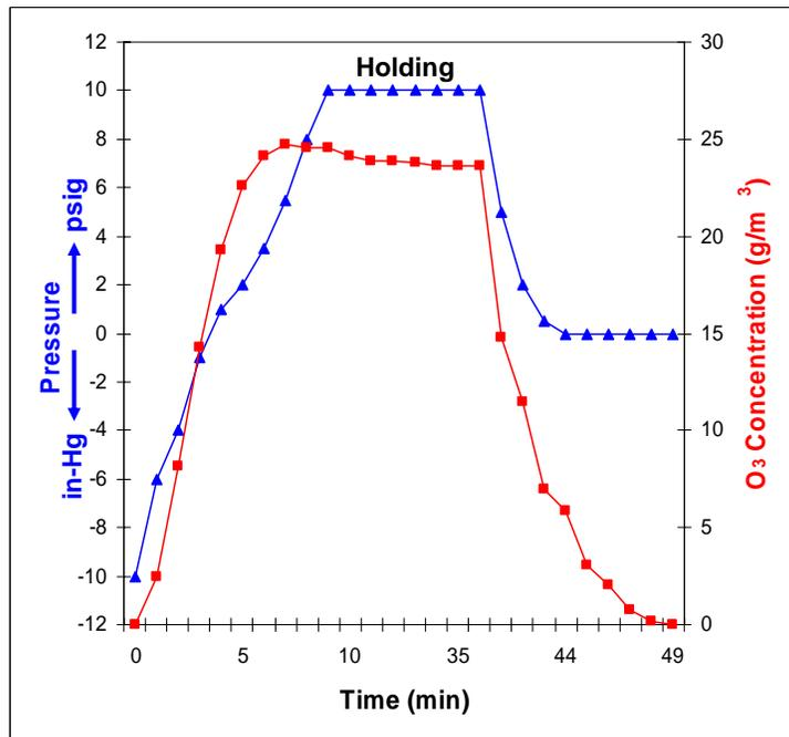
Figure C.9. Changes in typical process parameters including vacuum (in. of Hg), pressure (psig), and ozone concentration (g/m<sup>3</sup>) during treatment of fruits inside the treatment vessel during short-term treatments.
