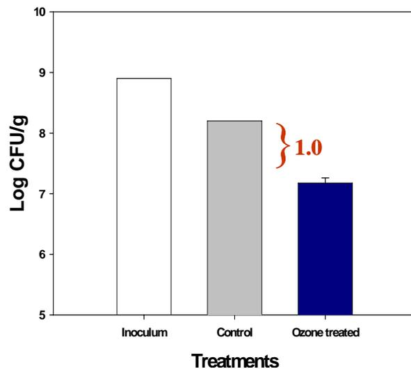
Figure C.8. Changes in population of *L. monocytogenes* OSY-328 on raspberries when treated with ~15 g/kg (20-21 g/m<sup>3</sup>) dry ozone at 10 psig for 30 min using Setup 2. Values are the average of duplicate samples of two experiments.
