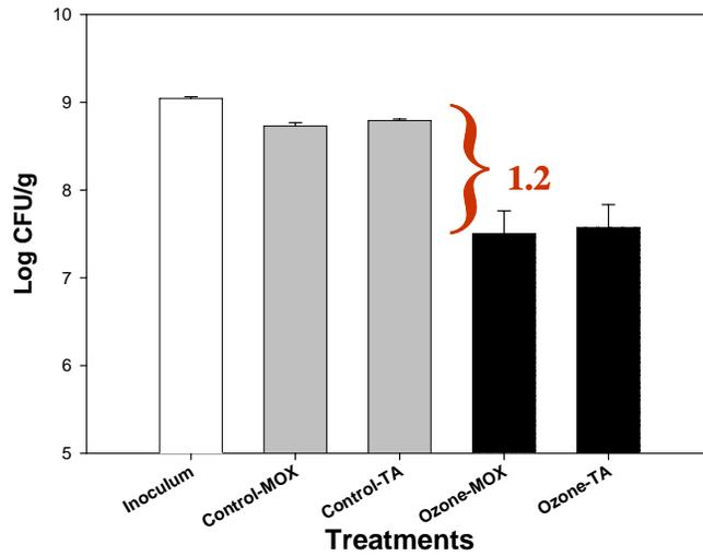
Figure C.3. Changes in population of *L. monocytogenes* OSY-328 on strawberries when treated with 60 g/kg (80 g/m<sup>3</sup>) moist ozone at 7.5 psig for 10 min using Setup 1. *Listeria* populations were enumerated on MOX agar and TA. Values are the average of duplicate samples of two experiments.
