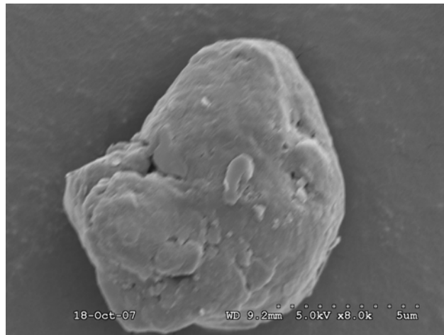
(c) Particles before sonication ( D \sim 5 - 10 \mu\text{m} )
