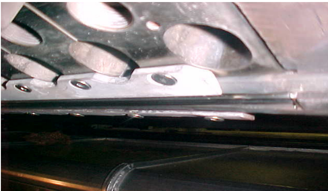
Figure 1.3 Lips on the die of the film manufacturing die used at DuPont – Circleville, OH
