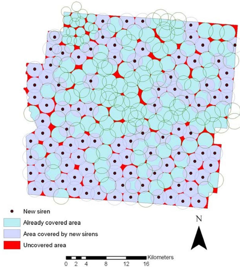
Figure 3.8. Siren configuration covering at least 95% of Franklin Co.
