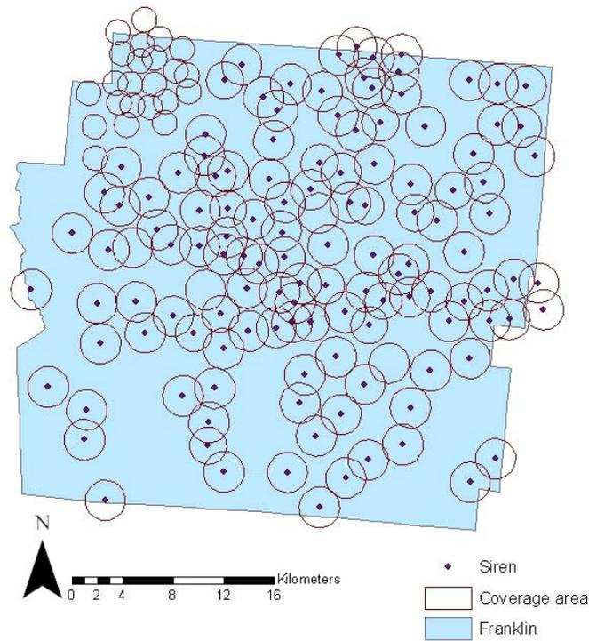
Figure 3.4. Existing warning siren coverage in Franklin Co., Ohio.
