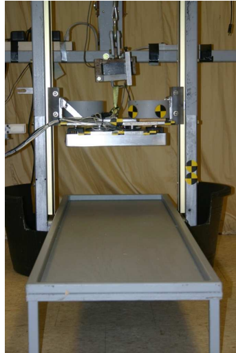
Figure 4.5: Drop tower modified for PMHS full body impact test
