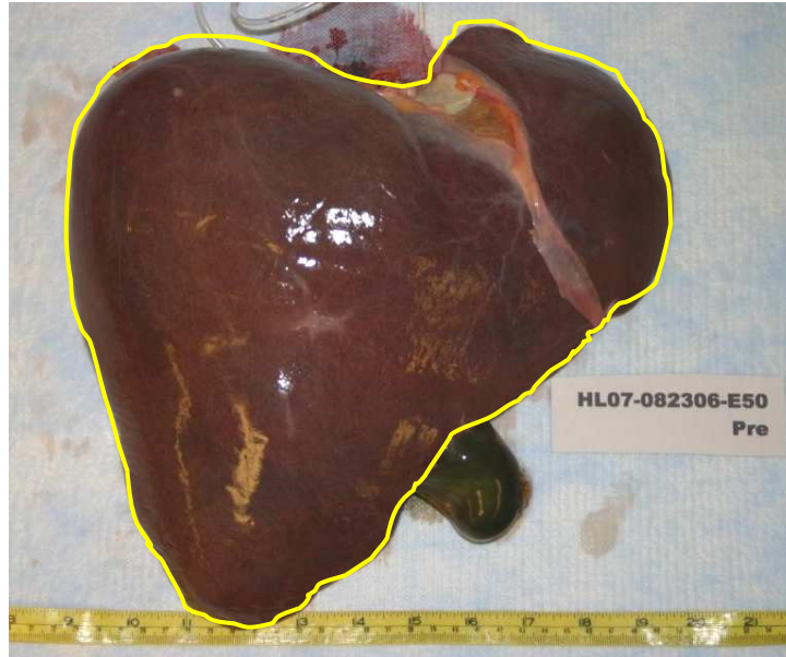
Figure 4.9: Pre-test liver photo with free-hand outline for area calculation using image analysis software
