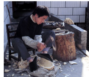
Figure 54: Hollowing the back of the woodblock
