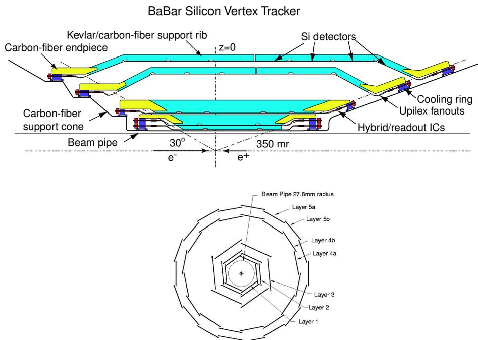
Figure 2.6: The longitudinal section (top) and the transverse view (bottom) of the Silicon Vertex Tracker in the *BABAR* detector.
