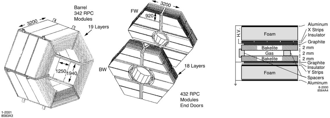
Figure 2.12: Barrel sector (left) and forward (FW) and backward (BW) endcaps, cross-section of the RPC (right).
