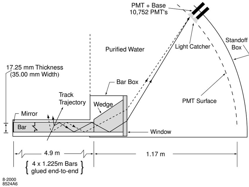
Figure 2.9: Schematics of the DIRC fused silica radiator bar (gray) and imaging region (the PMT Surface and the Standoff Box).
