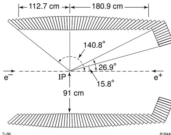
Figure 2.11: Longitudinal cross-section of the EMC.
