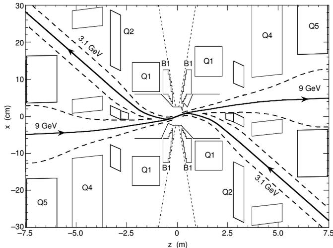
Figure 2.2: PEP-II interaction region where the electron (9 GeV) and positron (3.1 GeV) beams collide inside the *BABAR* detector. Bending (“B”) and focusing quadrupole (“QD”) magnets are responsible for the head-on collision of the beams.
