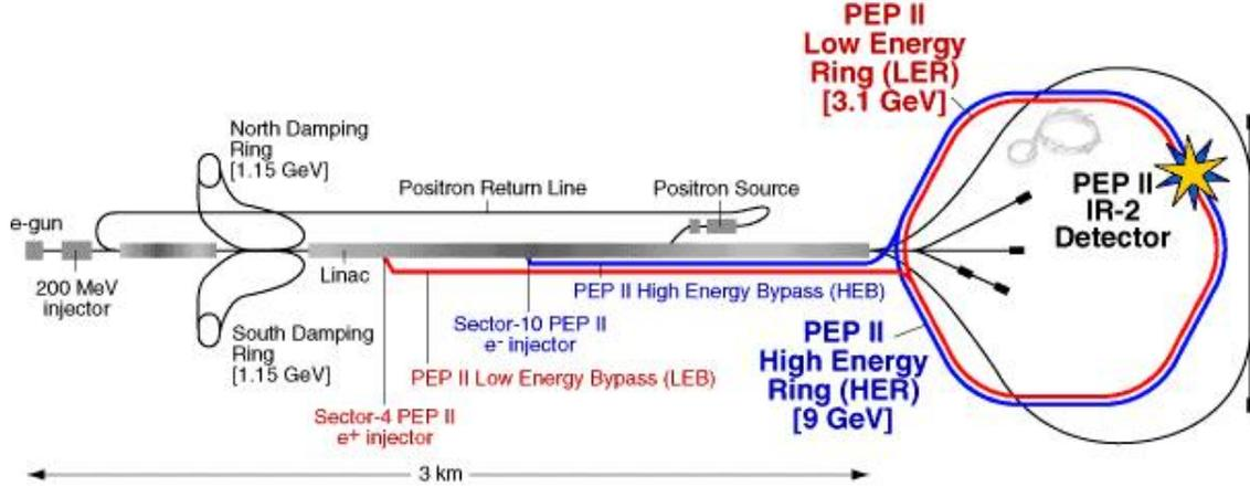
Figure 2.1: PEP-II facility and the linear accelerator layout.
